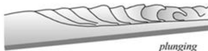
Figure 8 Plunging wave breaking is the most common type of breaking at the Holland coast. A lot of wave energy is released which causes an increased sediment transport gradient. (Image source: Holthuijsen (2007))
