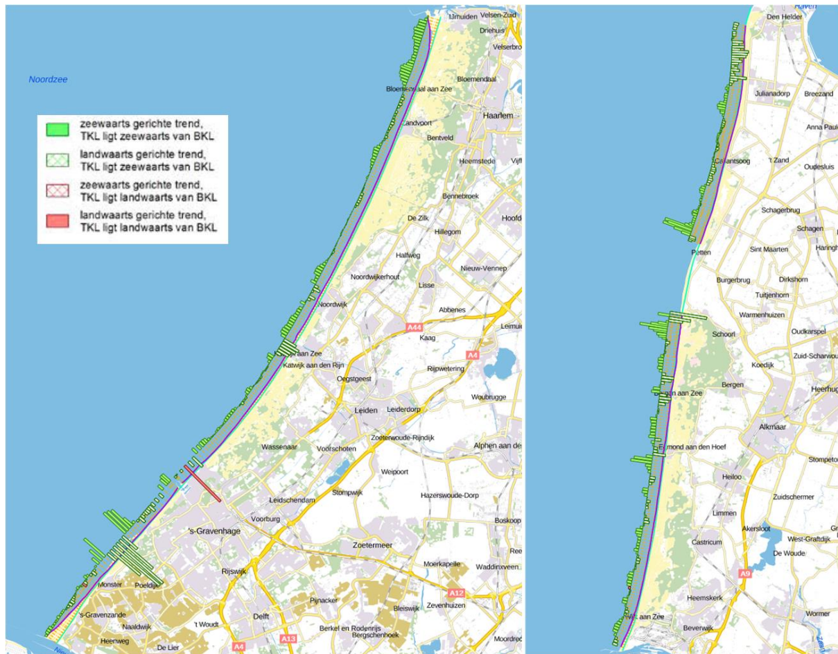
Figure 12 Annual measurements of the coastline position for the year 2018. The measurements are relative to the BKL. The left part shows the southern Holland coast between Hoek van Holland and IJmuiden. The right part shows the coastline between IJmuiden and Den Helder. (Image source: Rijkswaterstaat (n.d.))
