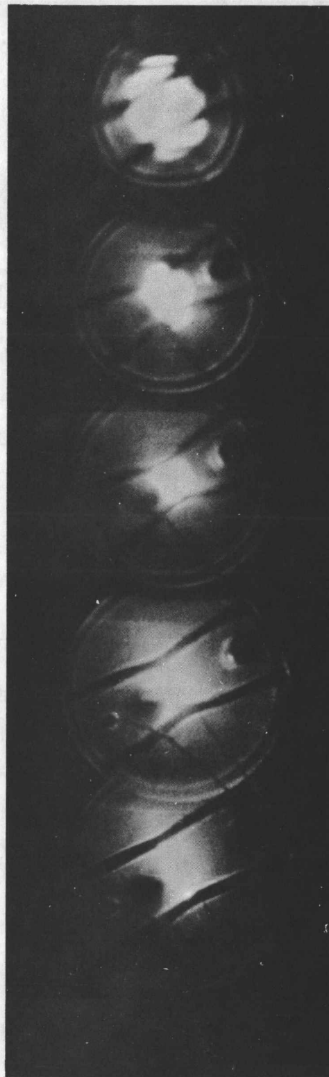
FIG 34 FRAMING CAMERA PICTURES OF DETONATION INITIATED BY AN EXPLODING WIRE
