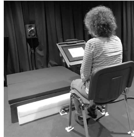
Fig. 4. Laboratory setup in AuraLab at Empa, with the graphical user interface of the experimental software application displayed on the screen and a porous floor absorber between the loudspeaker and the subject..
