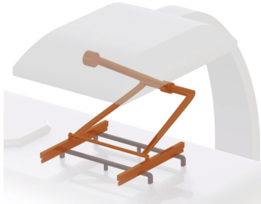
Figure 3.9: Concept of pantograph charging
