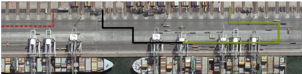
Figure 2.6: AGV movements during a discharge trip in black and green and during tanking in red
