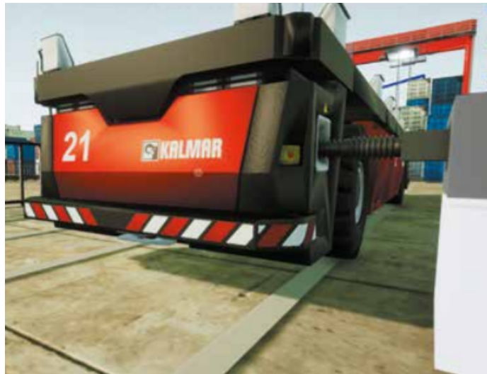
Figure 3.8: Kalmar FastCharge AGV Plug-in
