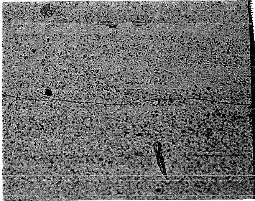
Figure 6.4: AA6061 specimen in self-made T6 condition perpendicular to the extrusion direction; magnification is 1000x
