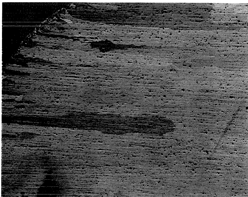
Figure 6.6: AA6061 in B condition, the extrusion direction is horizontal; magnification is 25x
