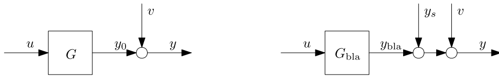
Fig. 4. The BLA represents a nonlinear system G using a LTI contribution G_{\text{bla}} , a stochastic nonlinear contribution y_s , and a noise source v .
