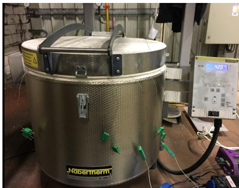
Figure 4.5: Nabertherm furnace used in life time tests.
