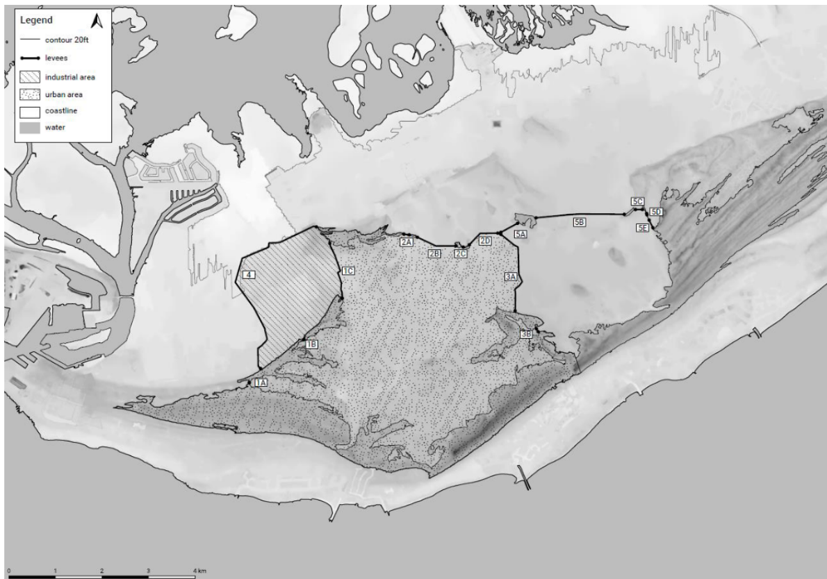
Figure 5.2: The design of the MDP “Grand Bahama after Hurricane Dorian; Interdisciplinary approach to Build Back Better”. Levees with their corresponding number and the 20 feet contours, surround the proposed collective protected area of Freeport which is divided in the industrial and urban areas [van der Hucht et al., 2021].
