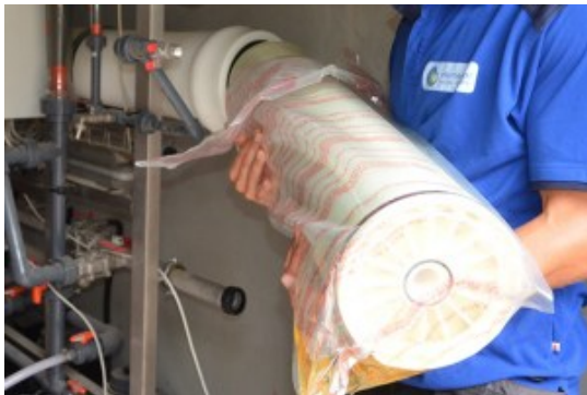
(c) [Reverse osmosis] is a membrane that rejects solutes and other particles while at the same time having a throughput (flux) of water. The high pressure used for this process is made by pumps which run on electricity.
