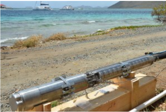
(a) [Intake pump] is where the water enters the pump intake system. The pressure provided by the pump distributes the water in the system. Most pumps have to be replaced yearly when used for salt water.
