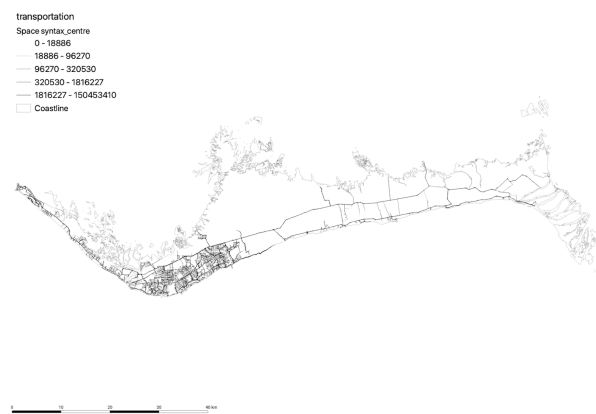
Figure 2.4: The space syntax analysis shows streets with the highest traffic (the darkest) on the island. Note, data from Grand Bahama Port Authority and Office of Coast Survey
