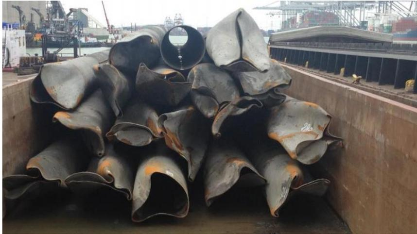
**Figure 3.4** Port of Rotterdam – Damaged pile toes (Bros et al., 2017)
