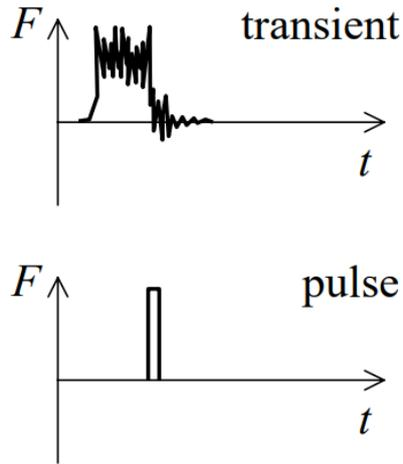
**Figure 2.4** Transient (above) and pulse (below) load
