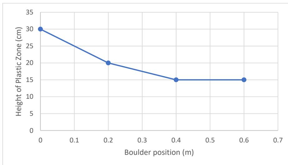
**Figure 5.33** Plastic zone height for each boulder position
