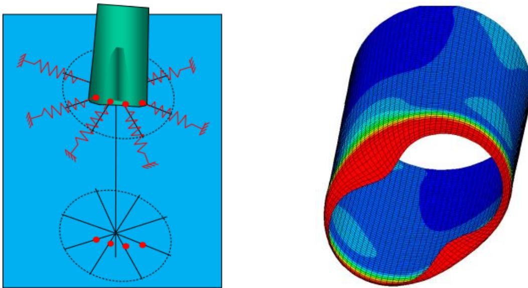
*Figure 3.14 BASIL - Soil represented as springs (left) and initial tip imperfection (right) (Randolph, 2018)*
