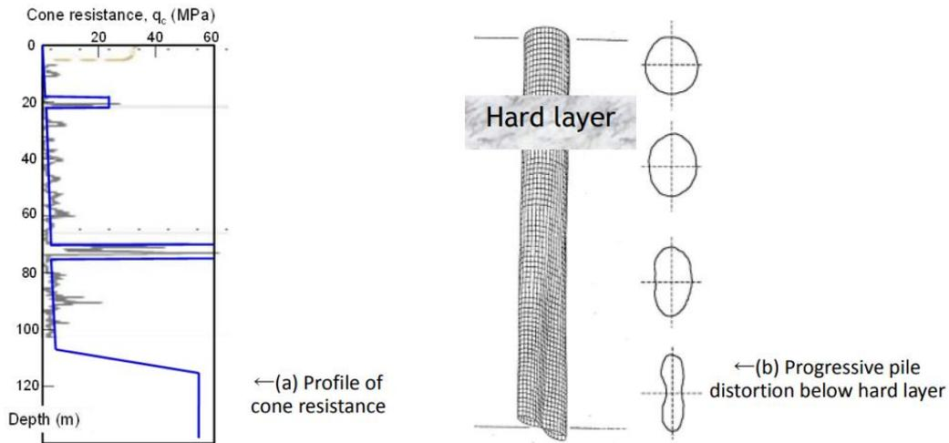
**Figure 3.6** Goodwyn A platform – Soil strength profile (left) and measured growth in pile distortion (right) (Randolph, 2018)
