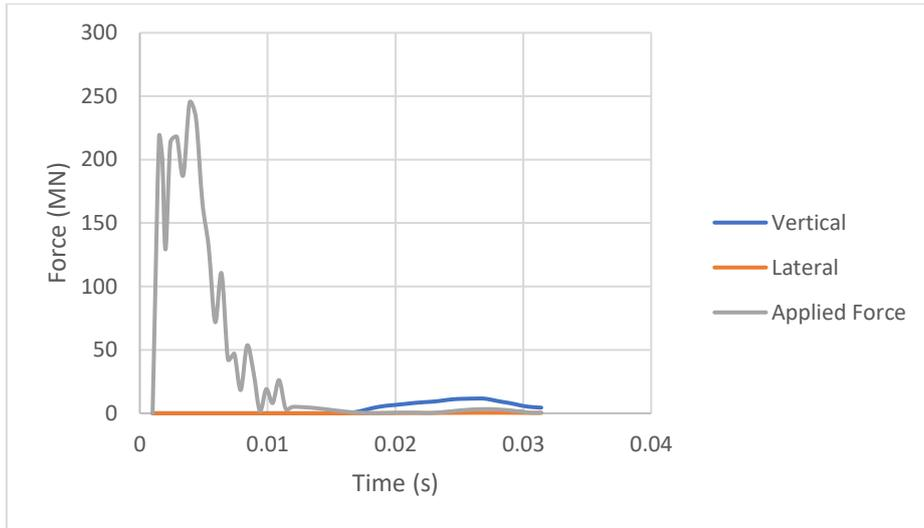
**Figure 5.31** Applied force, vertical and lateral reaction force – central (0 m) impact
