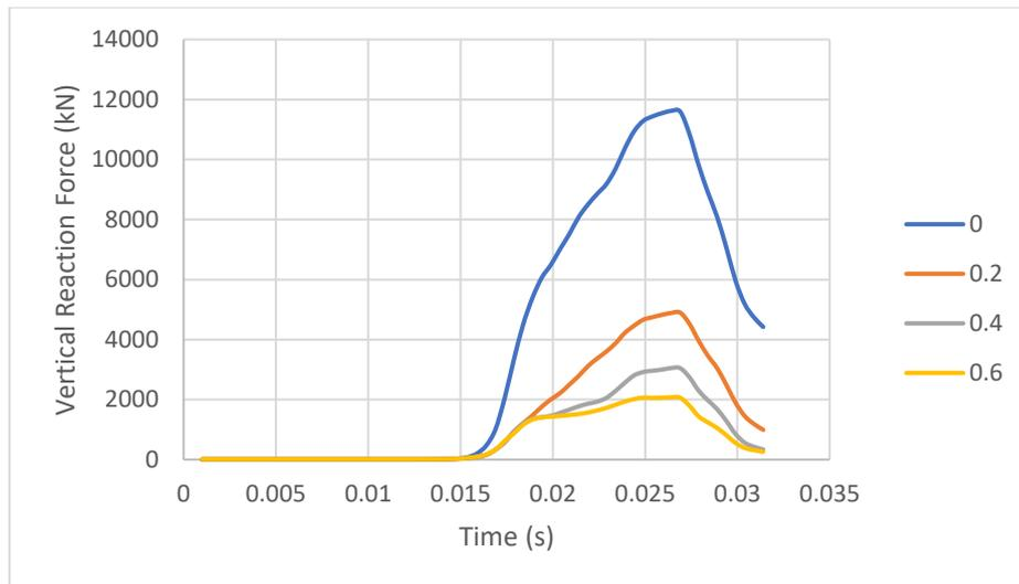
**Figure 5.28** Vertical reaction force at the boulder for different impact orientations
