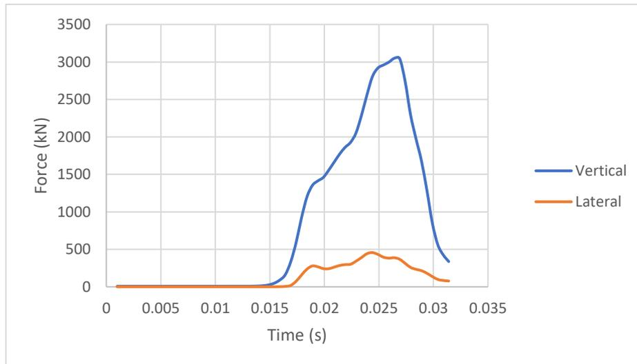
**Figure 5.30** Vertical and lateral reaction force on the boulder – eccentric (+0.4 m) impact
