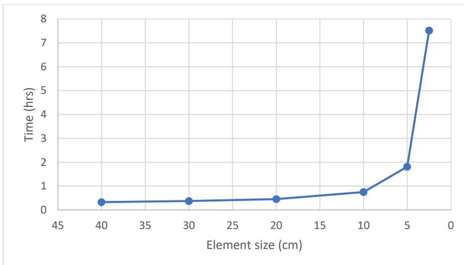
**Figure 5.14** Analysis time for different bottom mesh sizes
