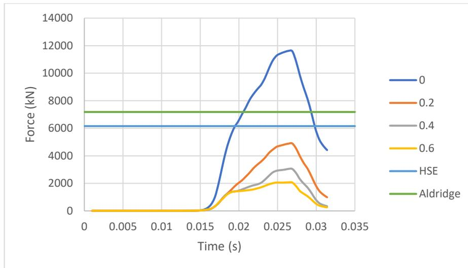
**Figure 5.50** Vertical reaction force at the boulder for different impact orientations and literature force limits
