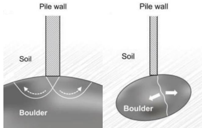
*Figure 3.1 Boulder failure mechanisms (Holeyman et al., 2015)*
