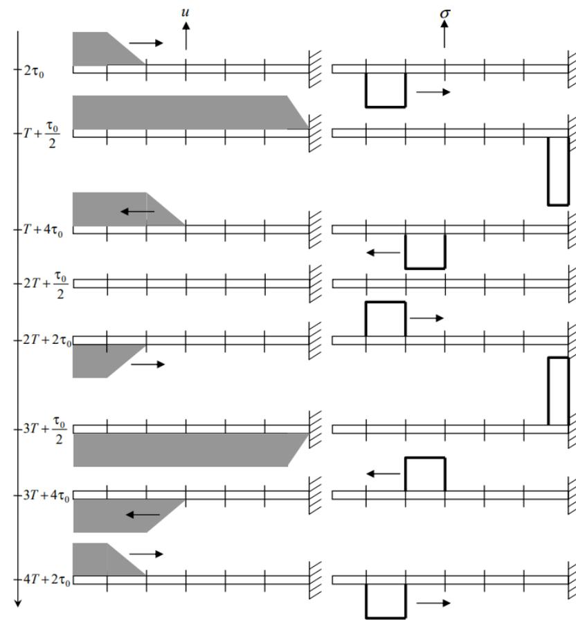
**Figure 2.2** Displacement (left) and corresponding stress (right) for a pulse propagating in a free-fixed pile
