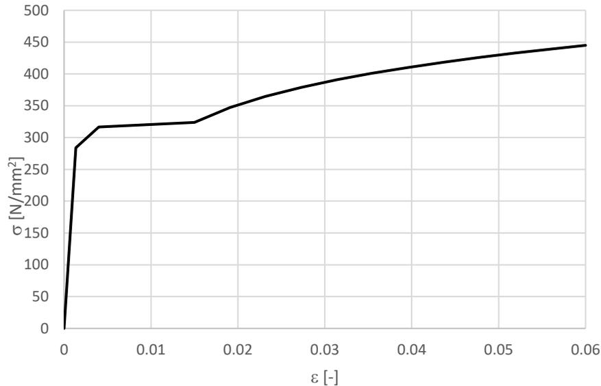
**Figure 4.1** S355 steel stress-strain curve (DNVGL-RP-C208, 2016)
