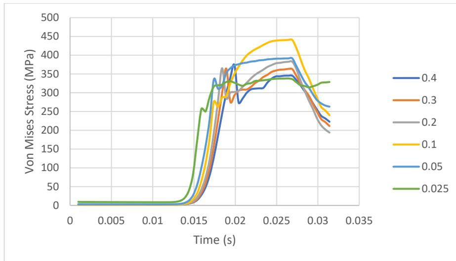
**Figure 5.7** Mesh sensitivity – Von Mises stress – Bottom node of the pile
