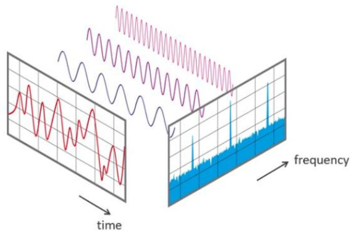
*Figure 2.7 View of a signal in the time and frequency domain [1]*
