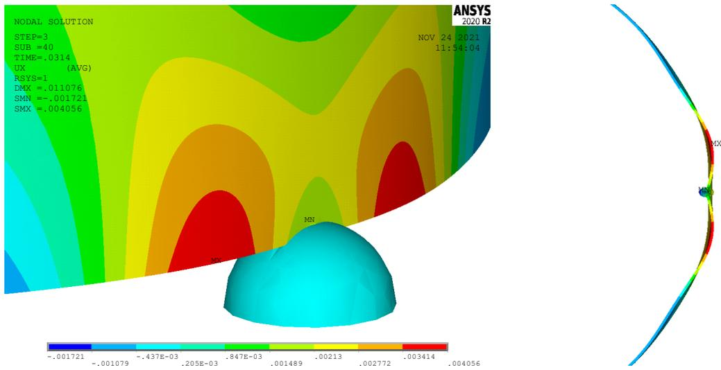
**Figure 5.34** Radial deformation - 3D side view (left, scaled by 20) and bottom view (right, scaled by 100) – Boulder position: 0 (central impact)
