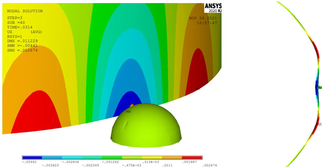
**Figure 5.37** Radial deformation - 3D side view (left, scaled by 20) and bottom view (right, scaled by 100) – Boulder position: +0.6
