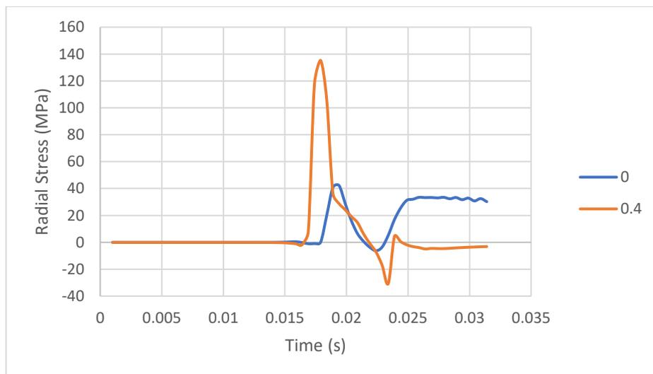
**Figure 5.25** Radial stress over time - Central (0 m) and eccentric (+0.4 m) impact
