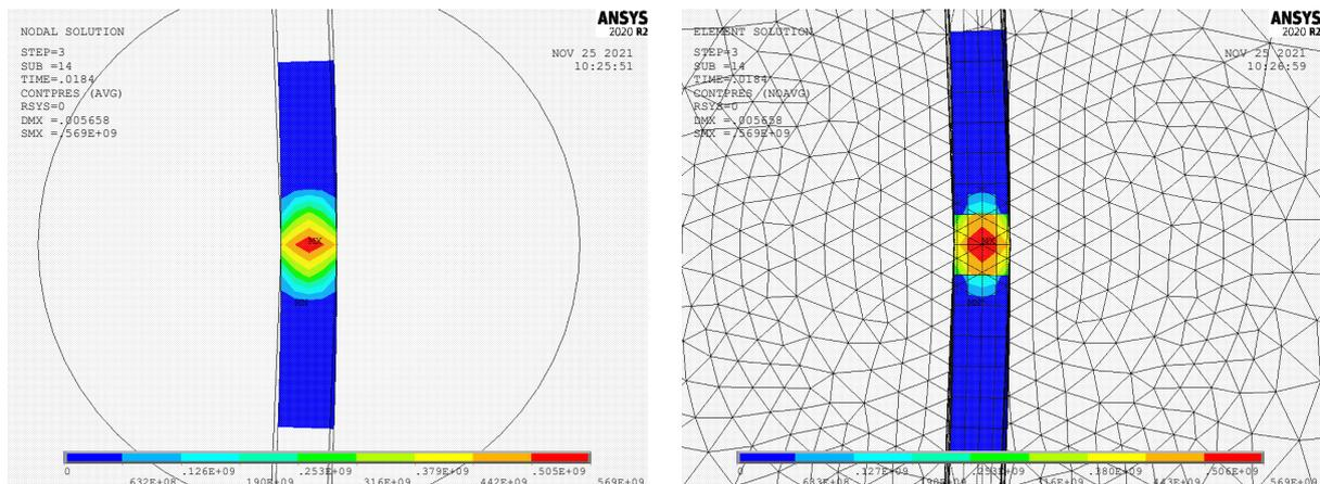
**Figure 5.19** Maximum contact pressure – Nodal (left) and element (right) solution – Central impact
