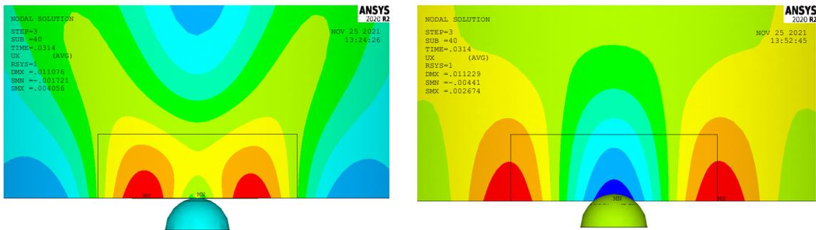
**Figure 5.41** Extent of radial deformations: central impact (left) and eccentric for +0.6 m boulder position (right), the black frame represents the pile circumference which corresponds to a 40° angle
