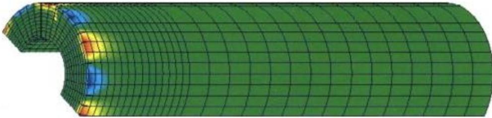
**Figure 2.8** Axial stress field of a thick cylindrical shell – solid elements
