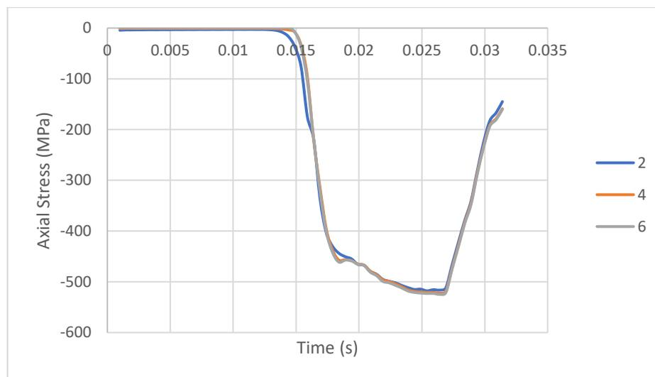
**Figure 5.15** Axial Stress at the bottom of the pile for 2,4 and 6 elements through the thickness
