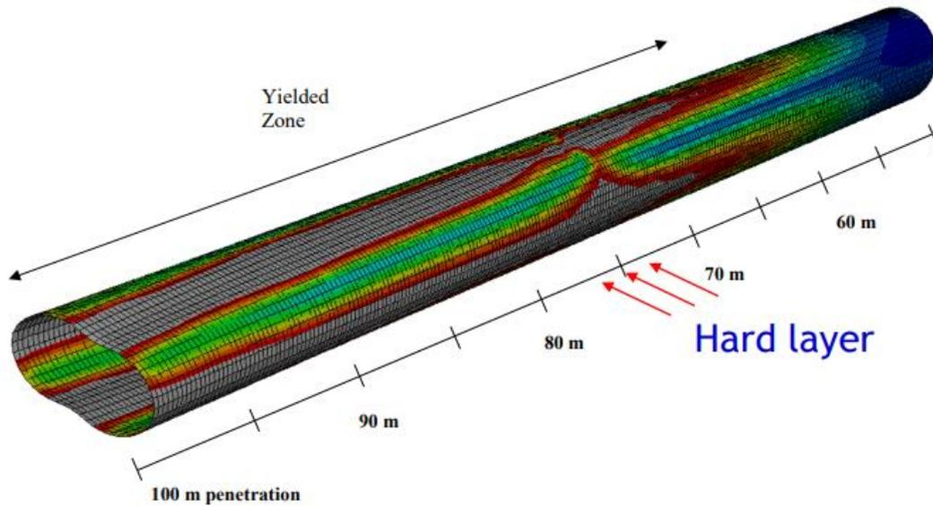
*Figure 3.15 BASIL – Plastic strains of a pile pushed 25 m beyond the hard layer (Randolph, 2018)*
