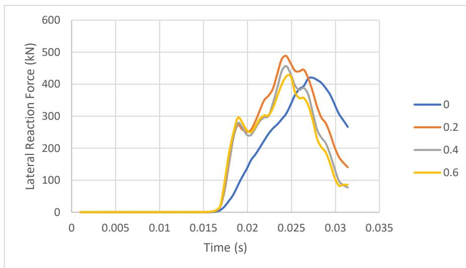
**Figure 5.29** Lateral reaction force at the boulder for different impact orientations
