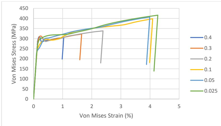
**Figure 5.11** Mesh sensitivity – Von Mises stress-strain relation – 10cm above pile tip
