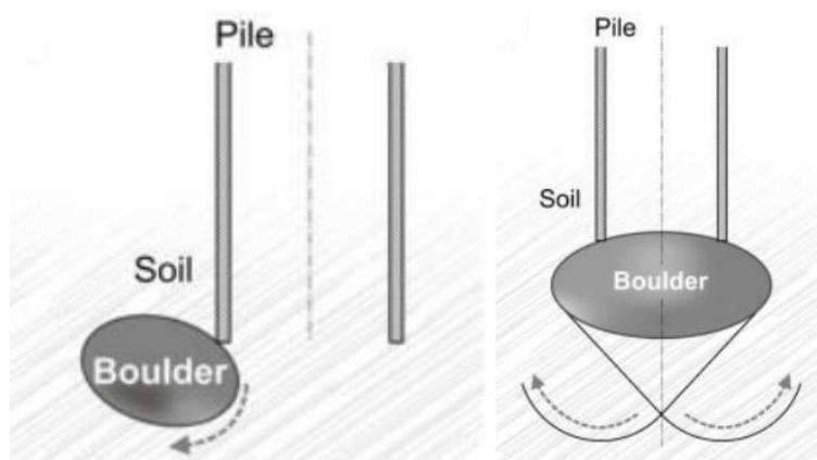
*Figure 3.2 Soil failure mechanisms (Holeyman et al., 2015)*
