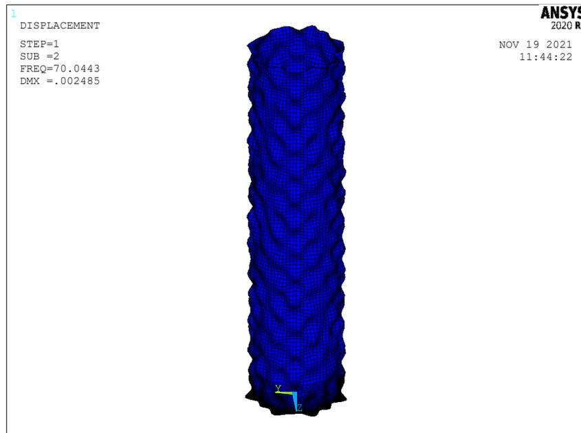
*Figure 5.45 Eigenmode for the 70 Hz frequency*
