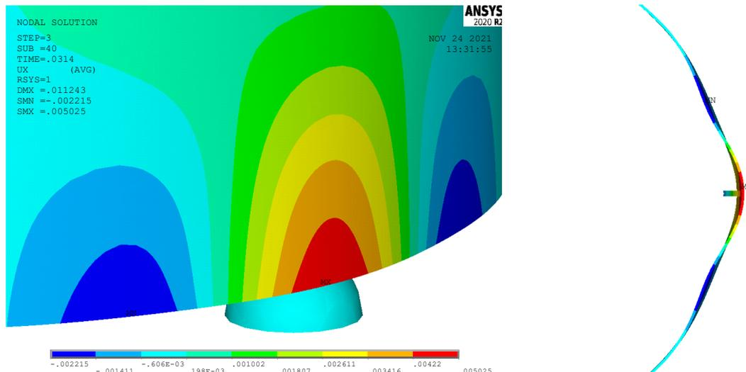
**Figure 5.40** Radial deformation - 3D side view (left, scaled by 20) and bottom view (right, scaled by 100) – Boulder position: -0.6
