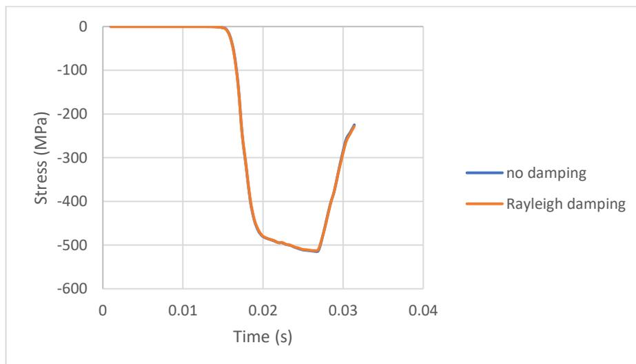
**Figure 5.47** Damping investigation - Axial stress at the pile tip over time
