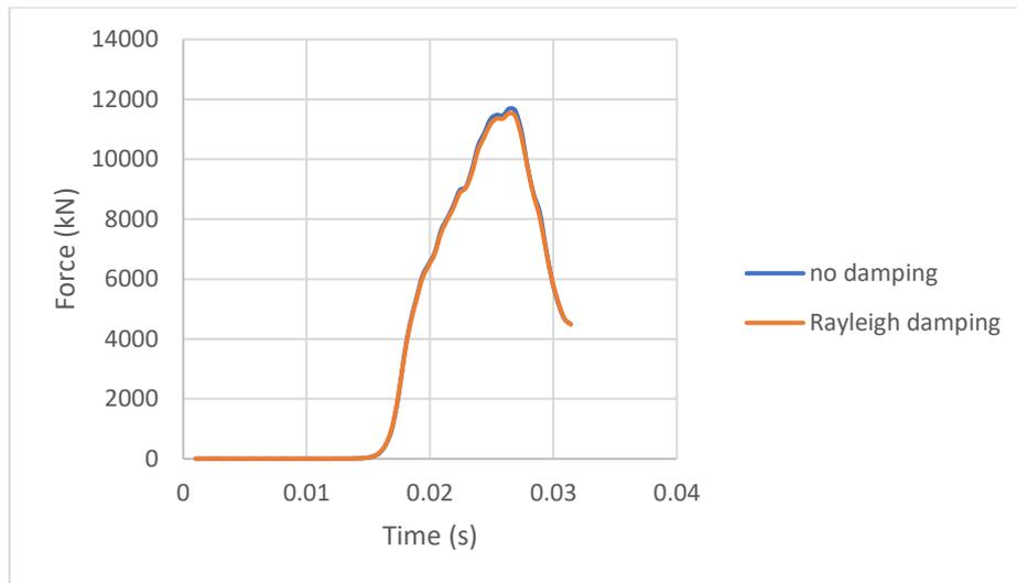
**Figure 5.48** Damping investigation – Vertical reaction force at the boulder
