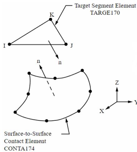
**Figure 4.6** TARGE170 geometry
