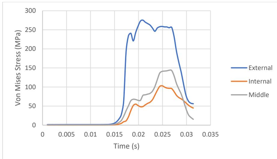
**Figure 5.22** Von Mises stress through the pile tip thickness, +0.4 m (Eccentric impact)
