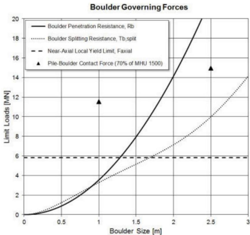
Figure 3.13 Limit loads of pile, boulder and soil as functions of boulder diameter (Holeyman et al., 2015)
