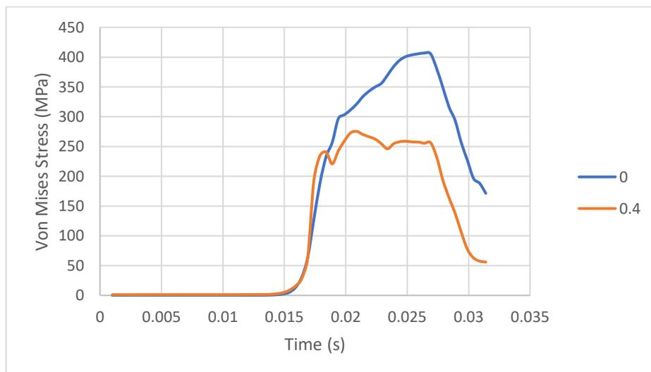
**Figure 5.23** Von Mises stress over time – Central (0 m) and eccentric (+0.4 m) impact
