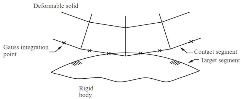
**Figure 4.5** Contact detection point at Gauss points
