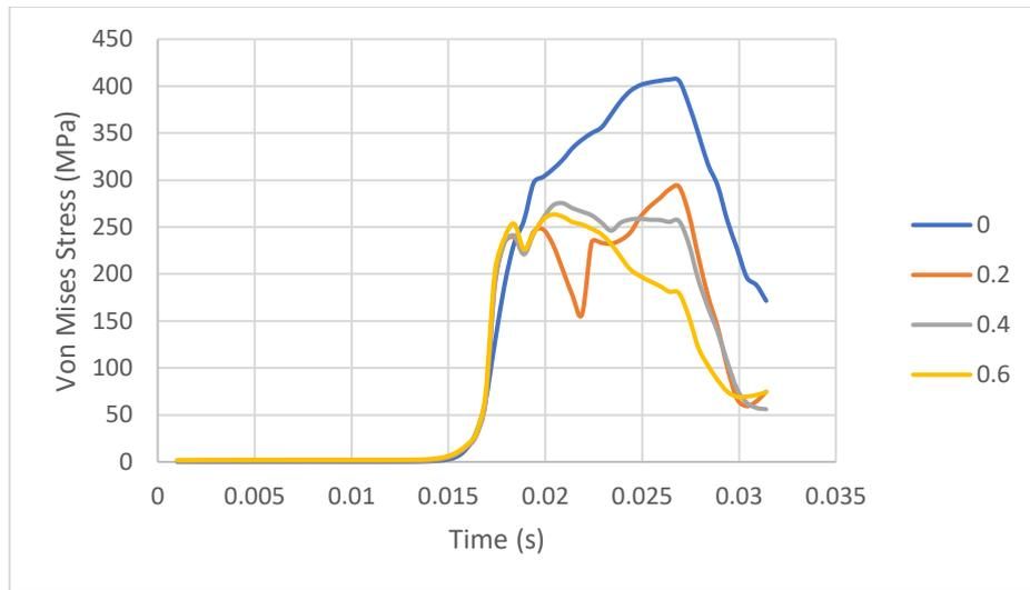
**Figure C.1** Von Mises stress over time at pile tip for central and eccentric (outside the pile wall) boulder positions
