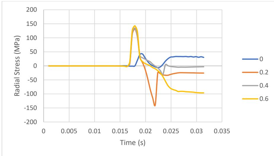
**Figure C.3** Radial stress over time at pile tip for central and eccentric (outside the pile wall) boulder positions
