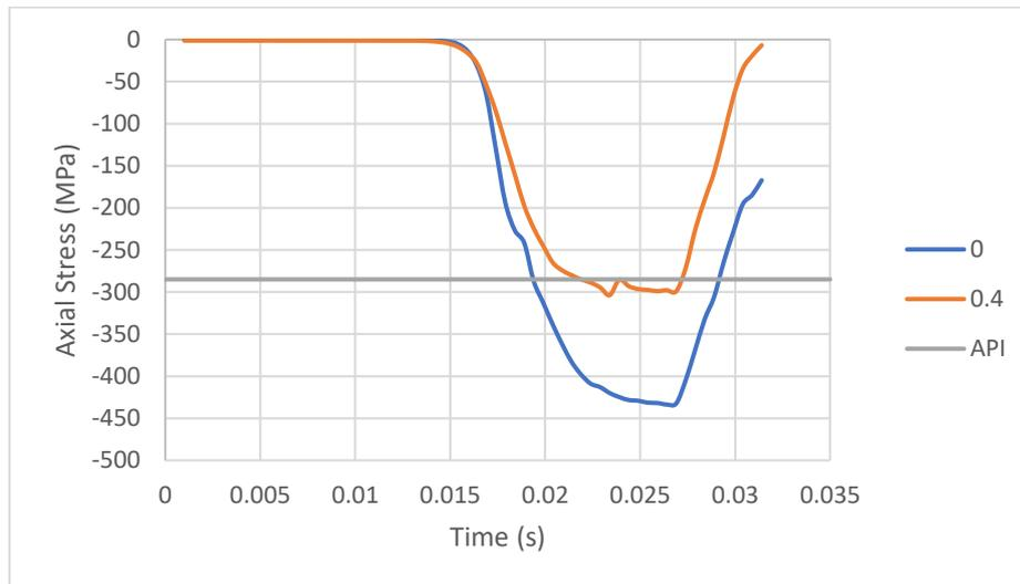
**Figure 5.49** Axial stress for central (0 m) and eccentric (+0.4 m) impact and API driving stress limit.
