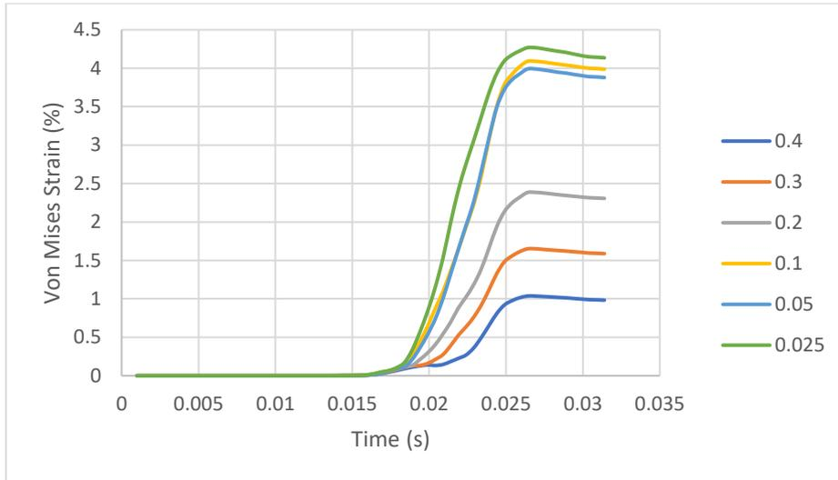
**Figure 5.10** Mesh sensitivity – Von Mises strain – 10cm above the pile tip
