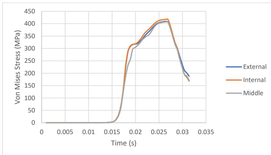
**Figure 5.21** Von Mises stress through the pile tip thickness, 0 m (Central impact)
