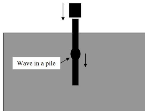
*Figure 2.1 Longitudinal wave in a pile*
