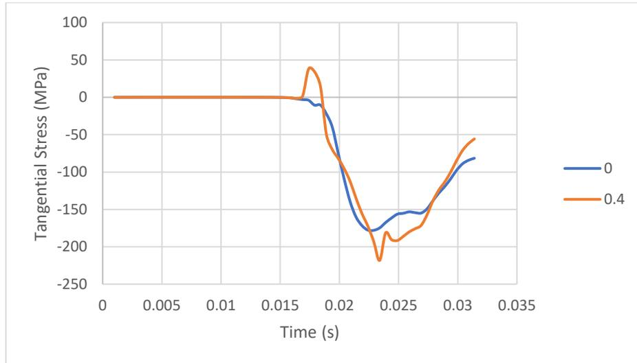
**Figure 5.26** Tangential stress - Central (0 m) and eccentric (+0.4 m) impact
