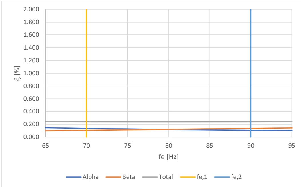
**Figure 5.46** Computed Raleigh damping for the selected range of monopile frequencies
