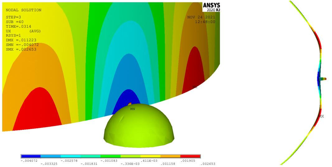
**Figure 5.36** Radial deformation - 3D side view (left, scaled by 20) and bottom view (right, scaled by 100) – Boulder position: +0.4
