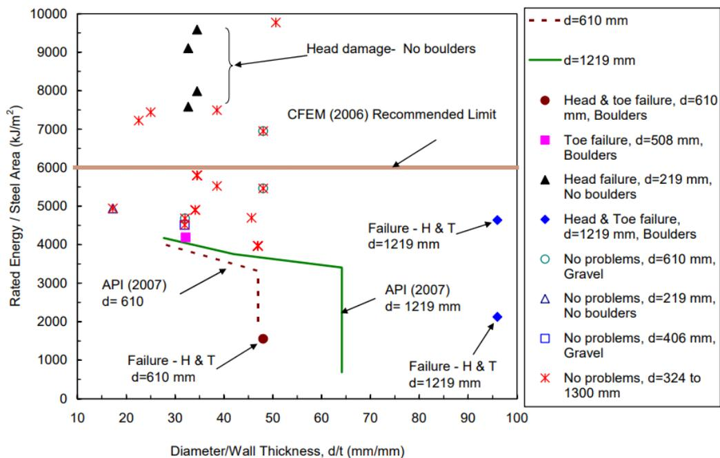
**Figure 3.8** Case studies for D/t ratio versus hammer energy showing API and CFEM recommended limits (Mostafa, 2011)
