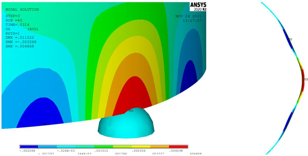
**Figure 5.38** Radial deformation - 3D side view (left, scaled by 20) and bottom view (right, scaled by 100) – Boulder position: -0.2
