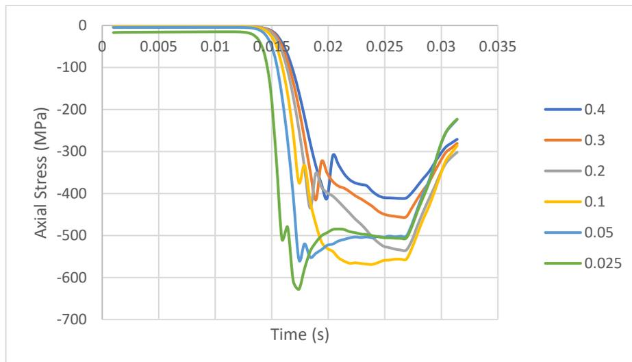
**Figure 5.8** Mesh sensitivity – Axial stress – Bottom node of the pile
