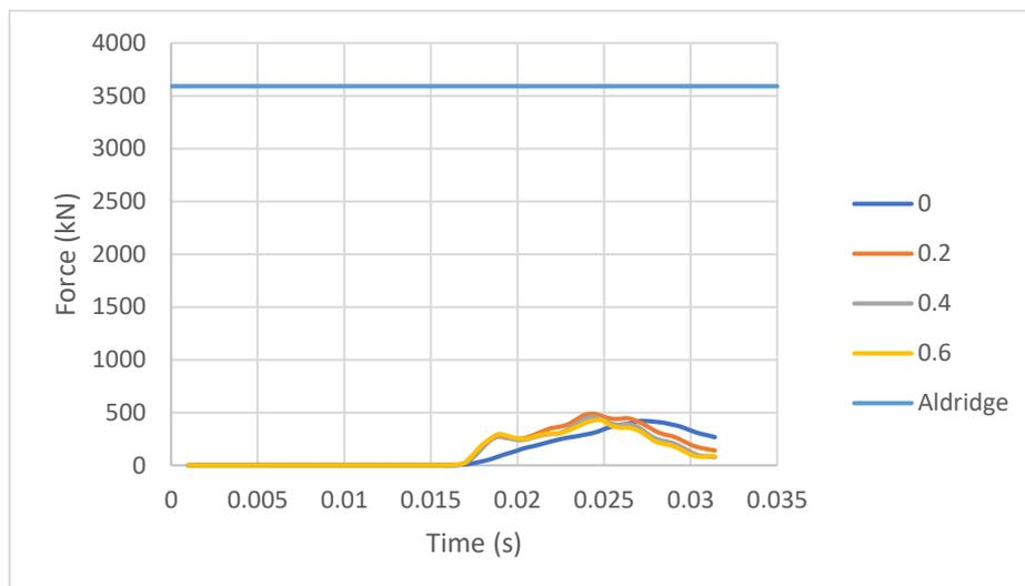
**Figure 5.51** Lateral reaction force at the boulder for different impact orientations and Aldridge's force limit
