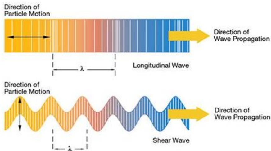
*Figure 2.3 Longitudinal and shear waves*
