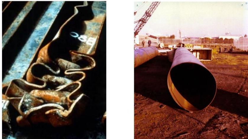
*Figure 3.3 Tip buckling of H-pile (left), Distortion of thin-walled tubular pile (right) (Randolph, 2018)*
