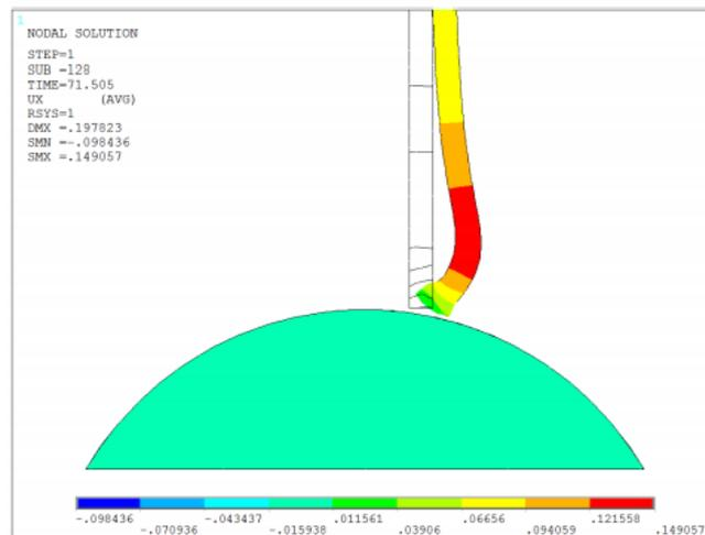
*Figure 3.16 Example of the resulting radial deformations at the pile tip (Jorna, 2018)*
