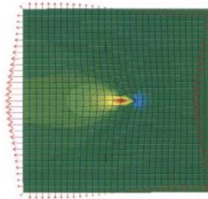
**Figure 2.10** Longitudinal normal stress field of a square plate
