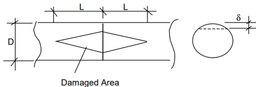
**Figure 3.11** Plan and section on damaged tubular, HSE (2001)
