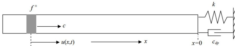
Figure 2.5 Local model for pile - soil interaction
