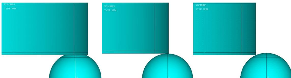
**Figure 5.20** Boulder positions: -0.4 m (left), 0 m-central (centre), +0.4 m (right)
