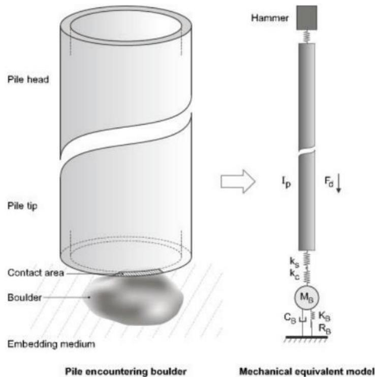
**Figure 3.12** Pile-boulder-soil model (Holeyman et al, 2015)
