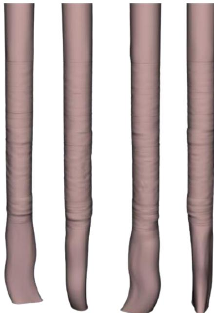
**Figure 3.7** Valhall platform – Typical distortion of lower part of piles (Randolph, 2018)
