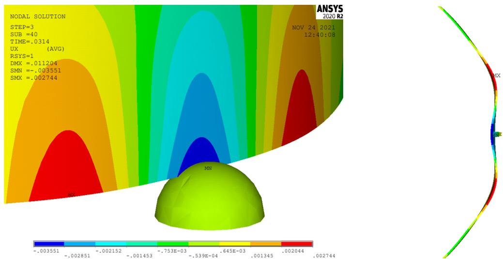
**Figure 5.35** Radial deformation - 3D side view (left, scaled by 20) and bottom view (right, scaled by 100) – Boulder position: +0.2
