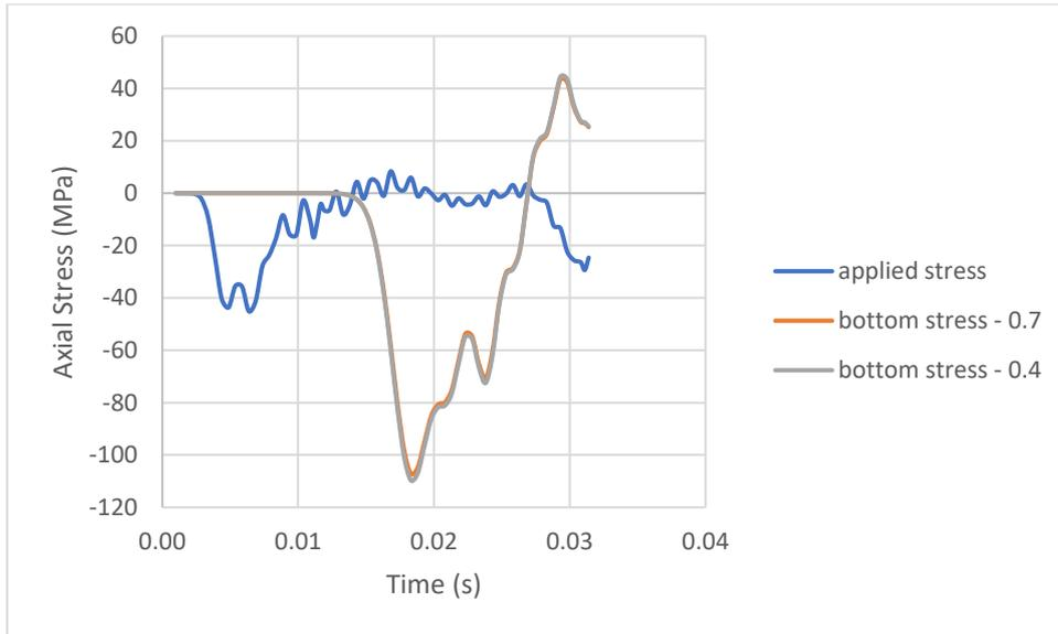
**Figure 5.3** Overall mesh size - Axial stress over time – Fixed pile
