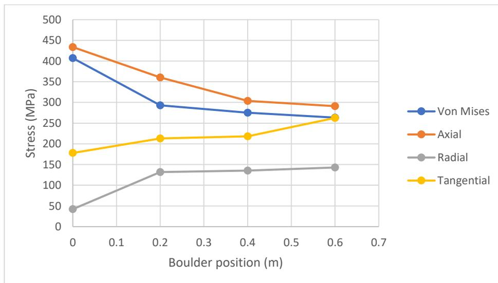
**Figure 5.27** Maximum stress values – Central (0 m) and eccentric (0.2, 0.4, 0.6 m) impact
