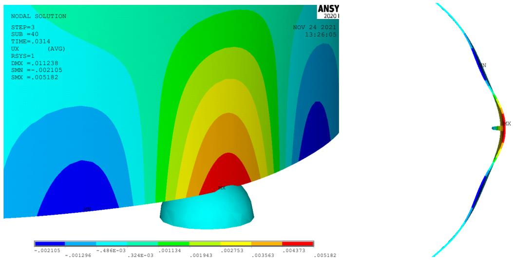
**Figure 5.39** Radial deformation - 3D side view (left, scaled by 20) and bottom view (right, scaled by 100) – Boulder position: -0.4
