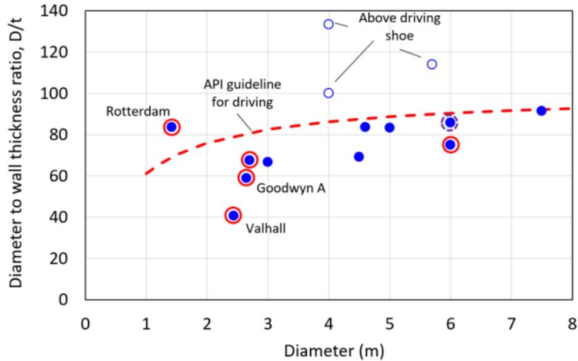
**Figure 3.9** Confirmed (red circle) and suspected (purple circle) extrusion buckling damage in open-ended pile geometries (Randolph, 2018)
