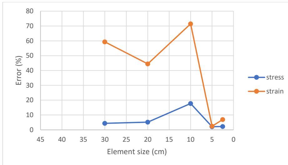
**Figure 5.12** Mesh sensitivity analysis – Convergence error of stress and strain
