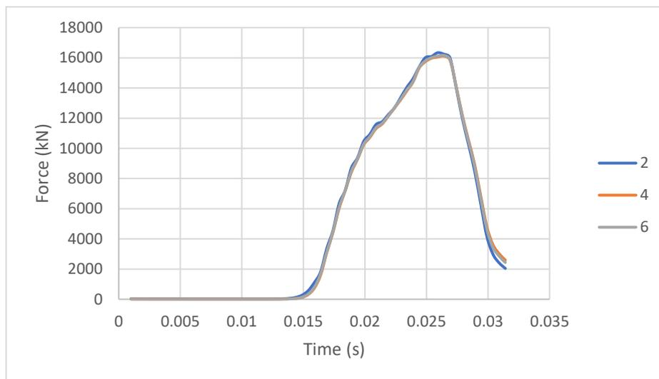
**Figure 5.17** Vertical reaction force at the boulder for 2, 4 and 6 elements through the thickness
