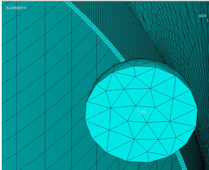
**Figure 5.18** Mesh view – 4 elements along through the pile thickness
