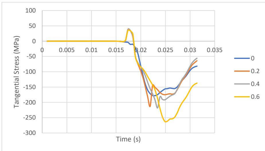
**Figure C.4** Tangential stress over time at pile for central and eccentric (outside the pile wall) boulder positions
