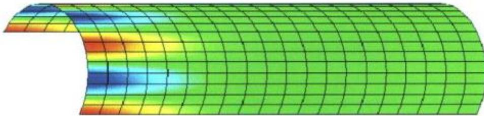
**Figure 2.9** Axial stress field of a thin cylindrical shell – shell elements
