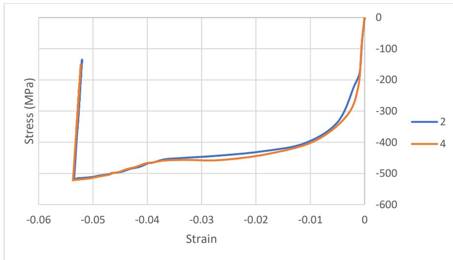
**Figure 5.16** Axial stress-Axial strain relation at the bottom of the pile for 2 and 4 elements through the thickness
