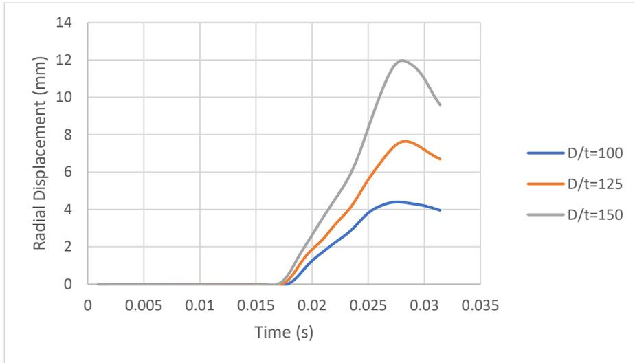
**Figure 5.42** *D/t ratio investigation – Radial displacement at the pile tip*
