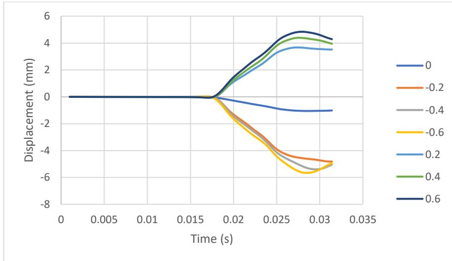
**Figure C.5** Pile tip radial displacement for central and eccentric (inside and outside the pile wall) boulder positions
