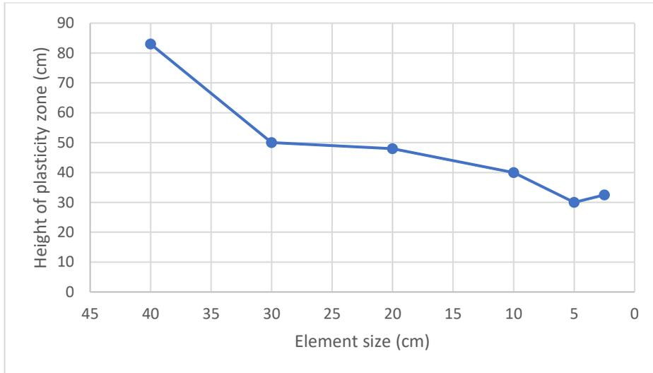
**Figure 5.13** Mesh sensitivity analysis – Height of the plasticity zone
