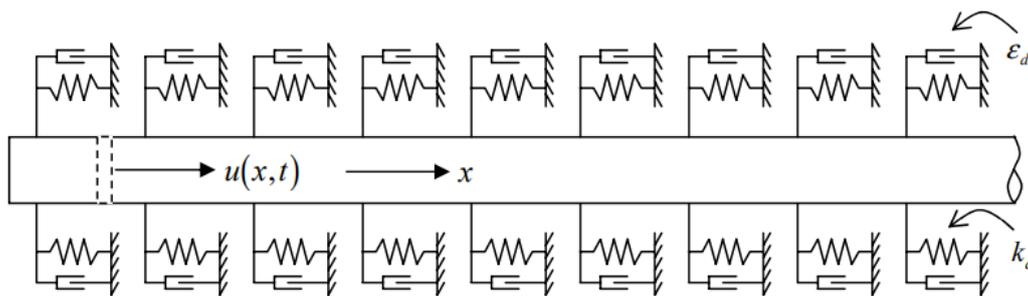
Figure 2.6 Distributed model for pile – soil interaction
