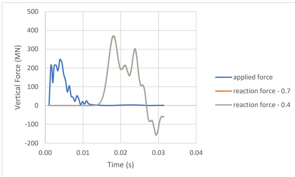
**Figure 5.4** Overall mesh size – Reaction force over time – Fixed pile
