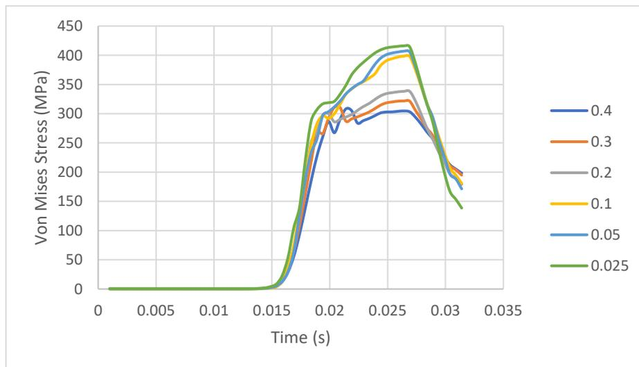
**Figure 5.9** Mesh sensitivity – Von Mises stress – 10cm above the pile tip
