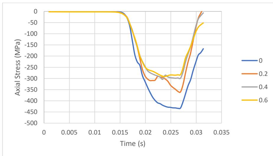
**Figure C.2** Axial stress over time at pile tip for central and eccentric (outside the pile wall) boulder positions
