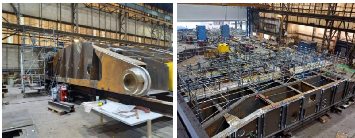
Figure 3.2: Construction of lock gates being produced at the Hollandia Infra production hall. Source: Hollandia Infra, 2021
