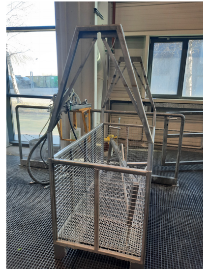
Tool to move components from one to another cleaning bath
