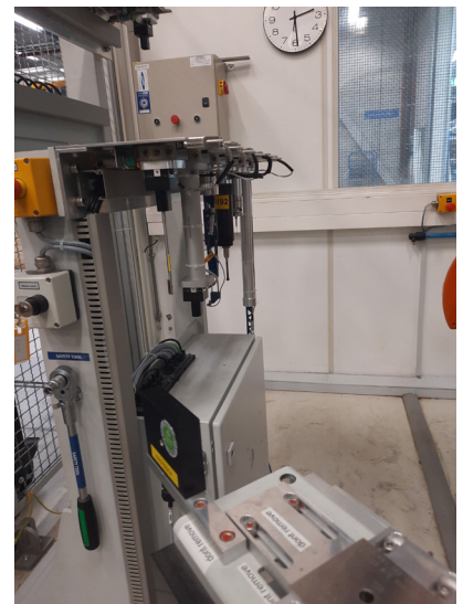
Robot used to identify cracks in the components
