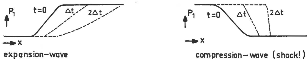
Fig. 16 Bedcomposition-waves using a bed-load formula including Egiazaroff's theory for \partial p_1/\partial x > 0 and \partial p_1/\partial x < 0 .
