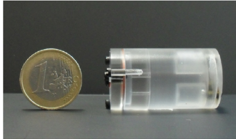
Figure 2-5: The SPECTIQ phantom: the down-sized version of the NU4IQ phantom (28)
