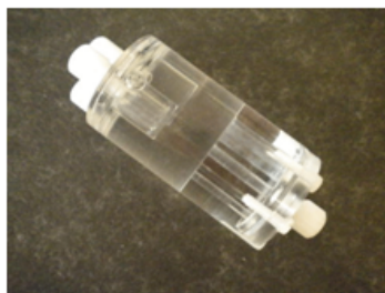
Figure 2-4: The NEMA NU 4 Image Quality (NU4IQ) phantom
