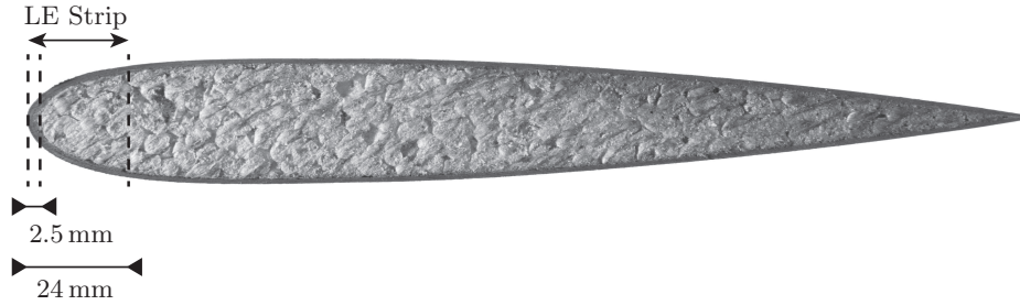
Figure 12: Cross-section of the experimental wing
