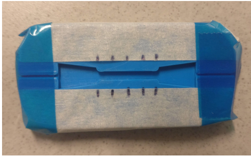
Figure 3.13: Dog-bone sectioning for microscope orientation
