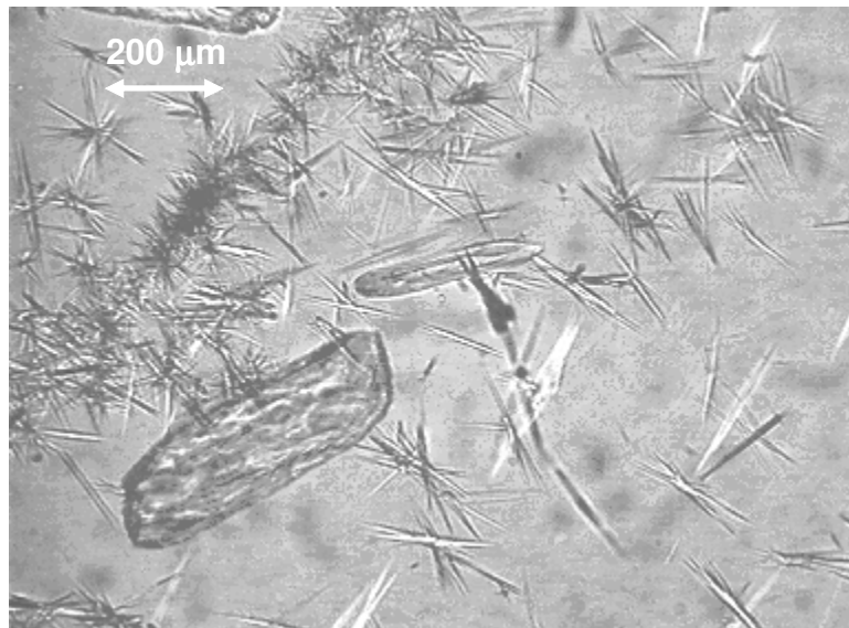
Figure 3-10: In-situ light microscope photograph taken during recrystallization of nahcolite ( \text{NaHCO}_3(\text{s}) = dissolving prism-shaped crystals) to wagscheiderite ( \text{Na}_2\text{CO}_3 \cdot 3\text{NaHCO}_3(\text{s}) = spherulitically growing, needle shaped crystals); bar = 200 micron
