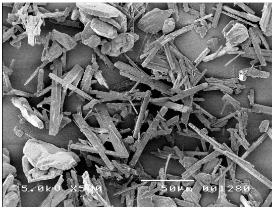
Figure 2-18: Sodium carbonate monohydrate from double recrystallization without impurity addition (bar = 50 micron)
