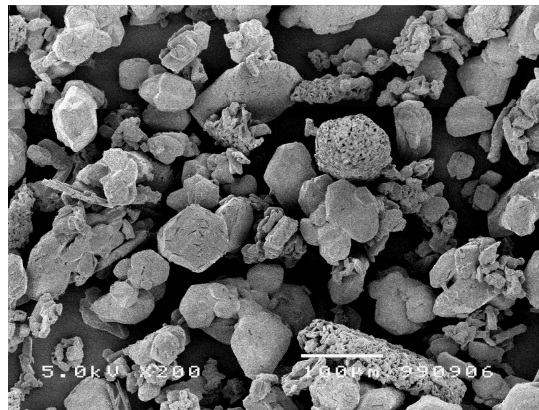
Figure 2-19: Sodium carbonate anhydrate from double recrystallization without impurity addition (bar = 100 micron)
