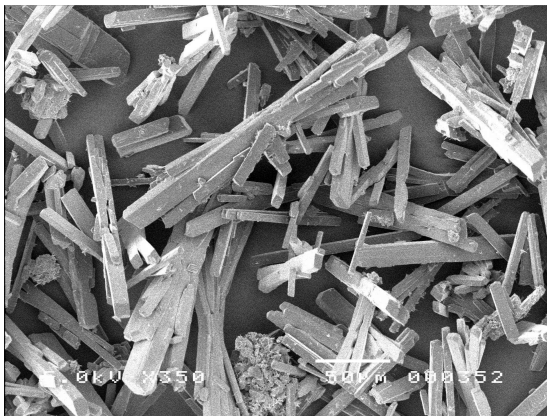
Figure 4-4: Mixed solvent trona formed from 70%-w ethylene glycol mixed solvent, bar = 50 micron
