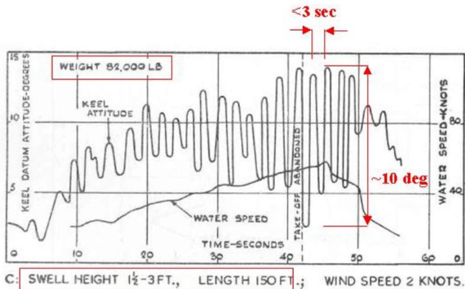
Figure 3.9: Effect of swell of length comparable or larger than aircraft length [11].
