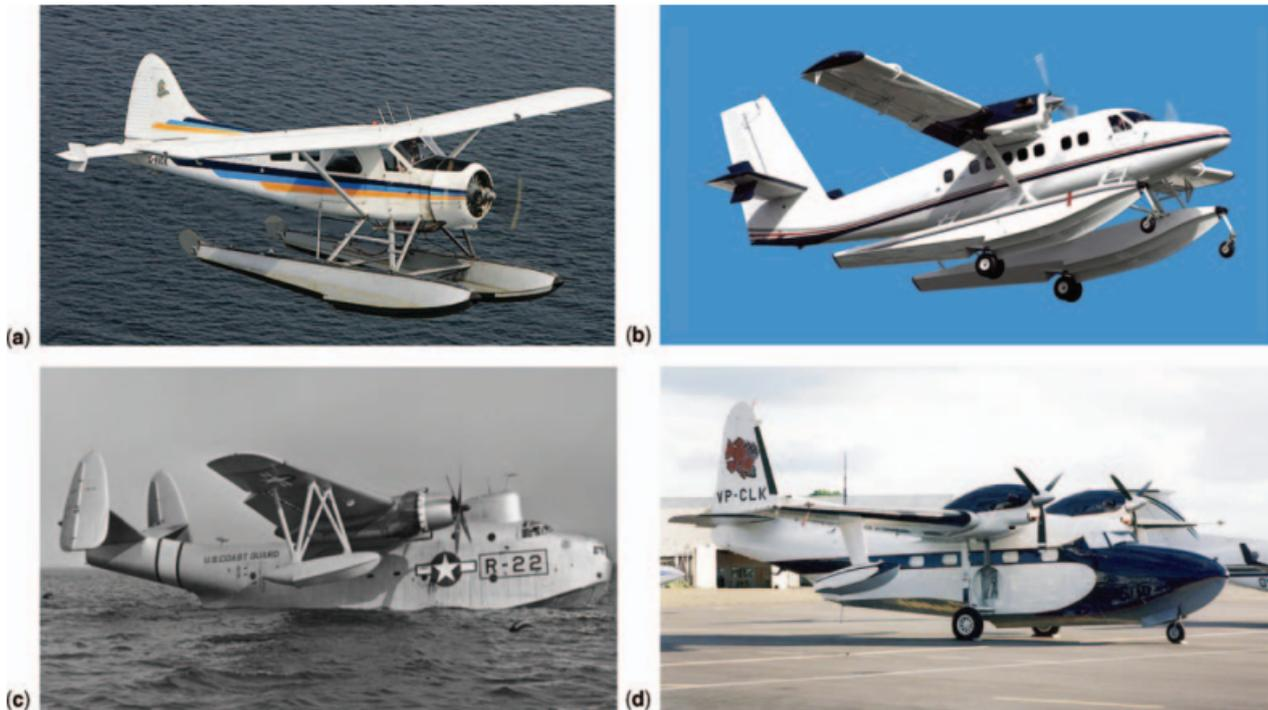
Figure 2.2: Seaplane main configurations: (a) A float-plane (de Havilland Beaver); (b) an amphibious float-plane (de Havilland Twin Otter); (c) a pure flying-boat (Martin PBM-5 Mariner); (d) an amphibious flying-boat (Grumman Mallard) [2].
