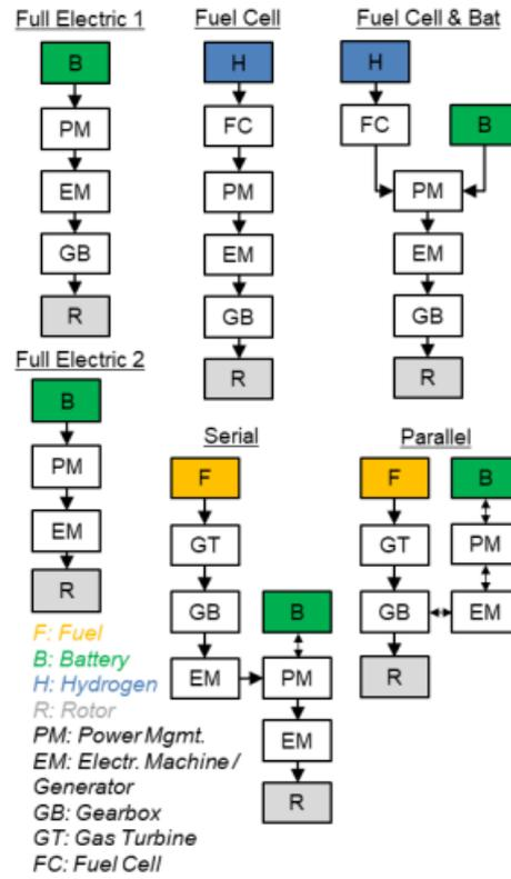
Figure 4.3: Simplified powertrain models [34].
