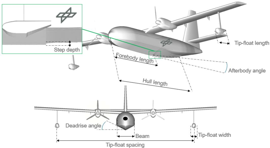
Figure 4.1: Flying-boats main geometrical parameters.
