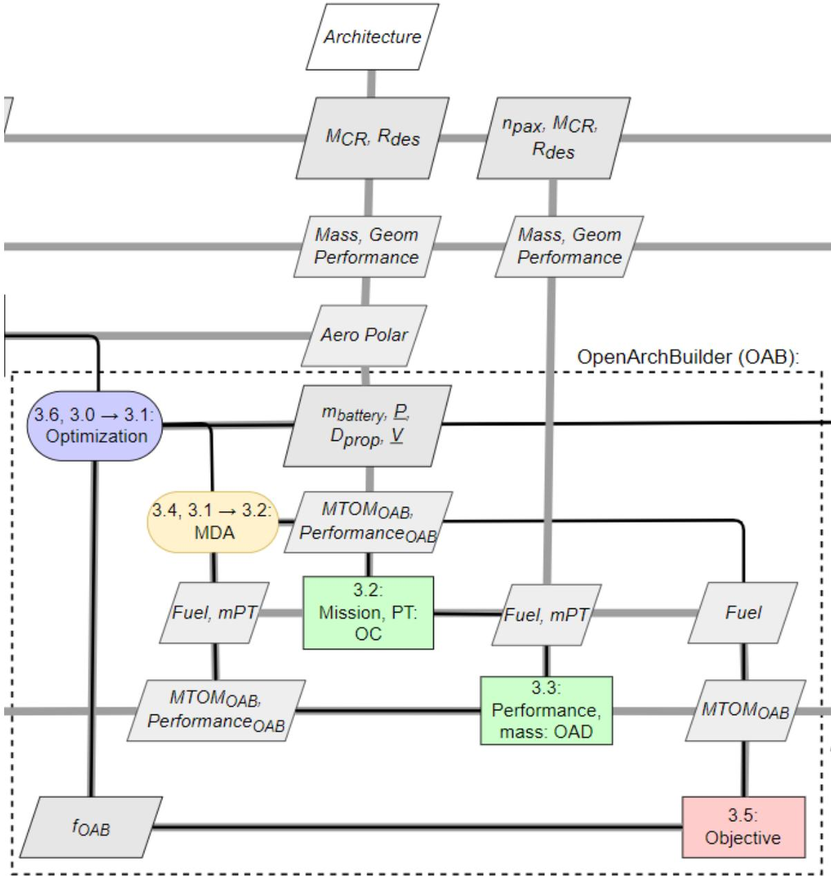
Figure A.3: Zoom in the XDSM diagram for the nested optimization loop in OpenArchBuilder
