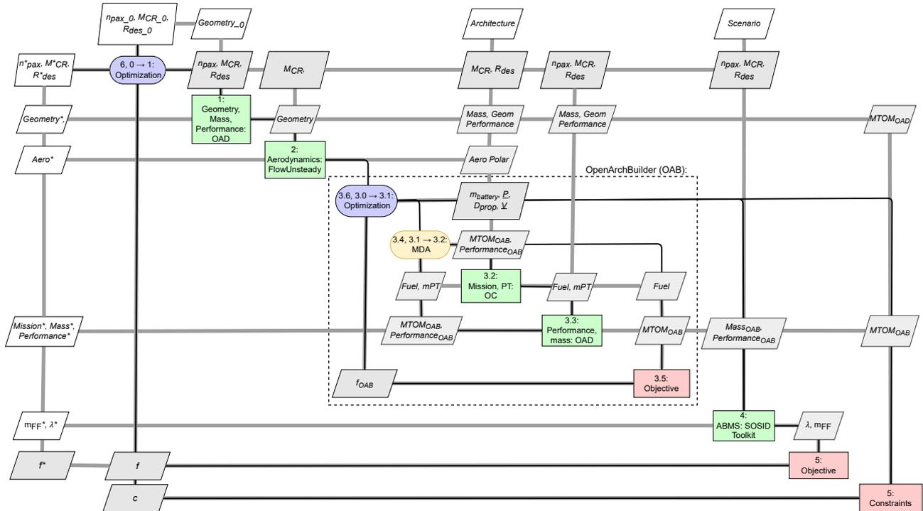
Figure 2 – XDSM diagram of the System of System-driven optimization problem
