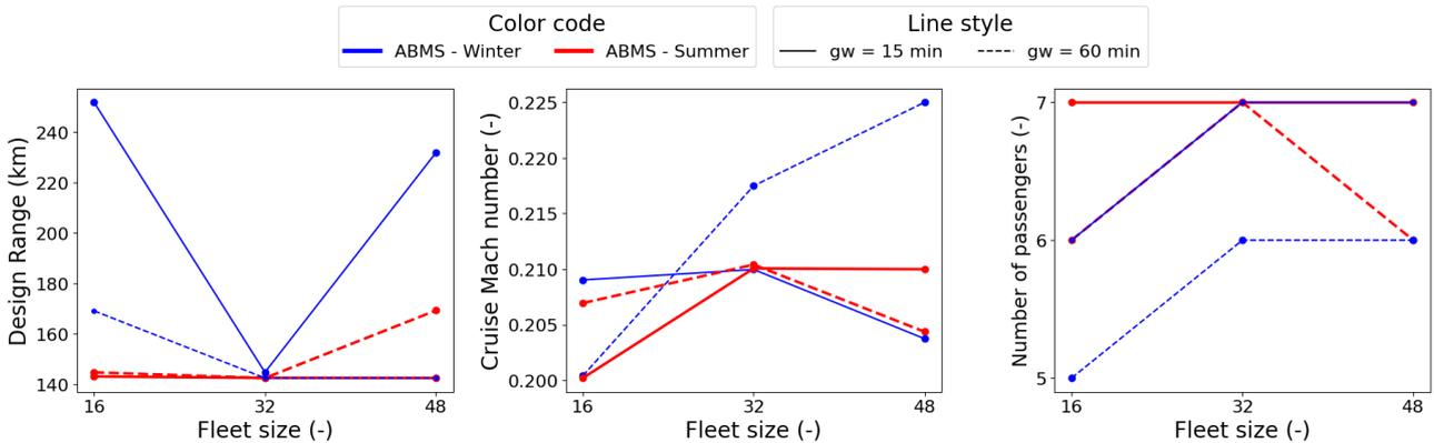
Figure 7 – Optimum seaplane design parameters in the different scenarios
