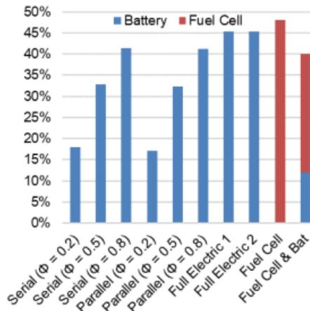
Figure 4.4: Battery and fuel cell mass fractions (w.r.t. MTOM) for UAM vehicles [34].
