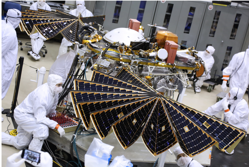
Figure 6.12: A deployment test of InSight's solar panels
