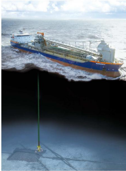
Figure 1.1: Van Oord's SRI vessel Nordnes covers a pipeline (Van Oord, 2016).
