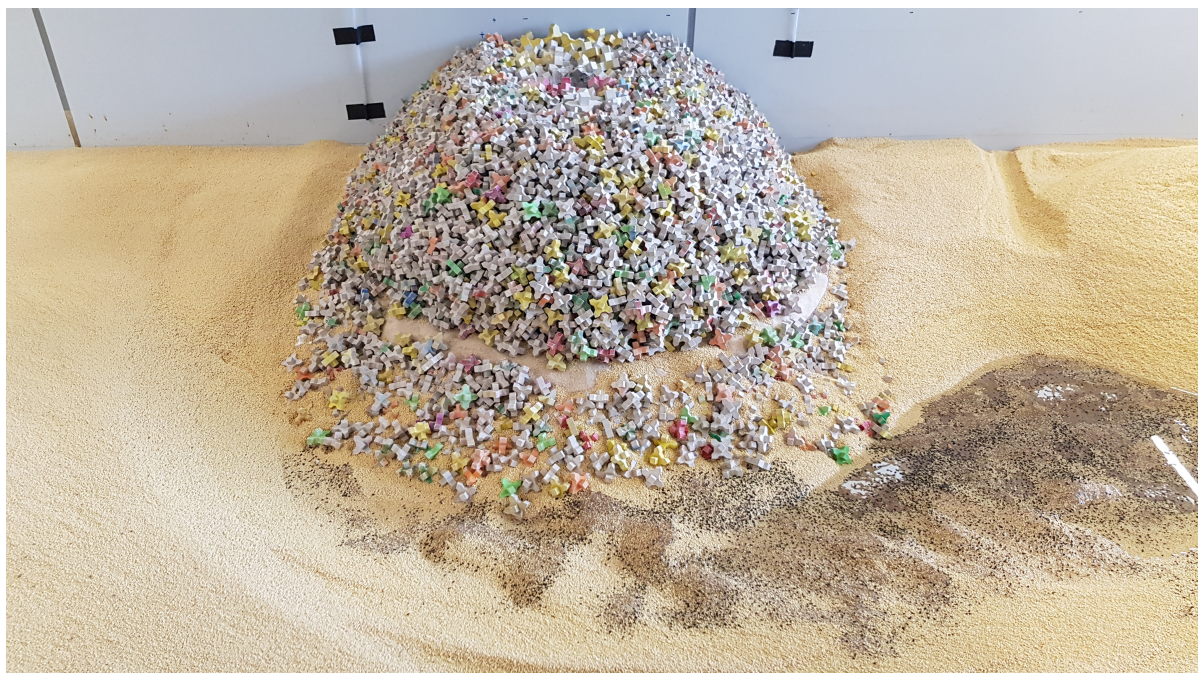
Scour formation around the flexible groyne head after experiment FG1
