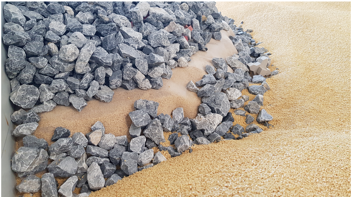
Scour at the upstream end of the stone structure in experiment SG1 where the geometrically closed filter protects the bed material from erosion
