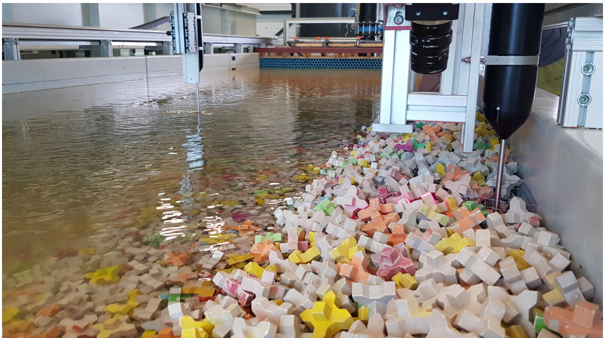
Installation of the velocimeters, the left one has side-looking probes and the one inside the structure is the Vectrino Profiler
