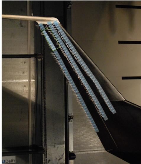
Figure 5.7: Tuft image of the outboard wing upper surface at  $\alpha = 25^\circ$ , including SF15 with  $\delta_{sf} = 40^\circ$  outlined in green.
