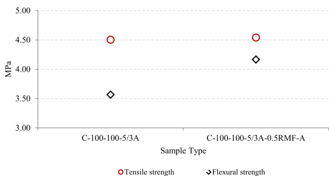
Fig. 9. Impact of mineral fibres on the tensile strength and flexural strength of recycled concrete at 28 days.
