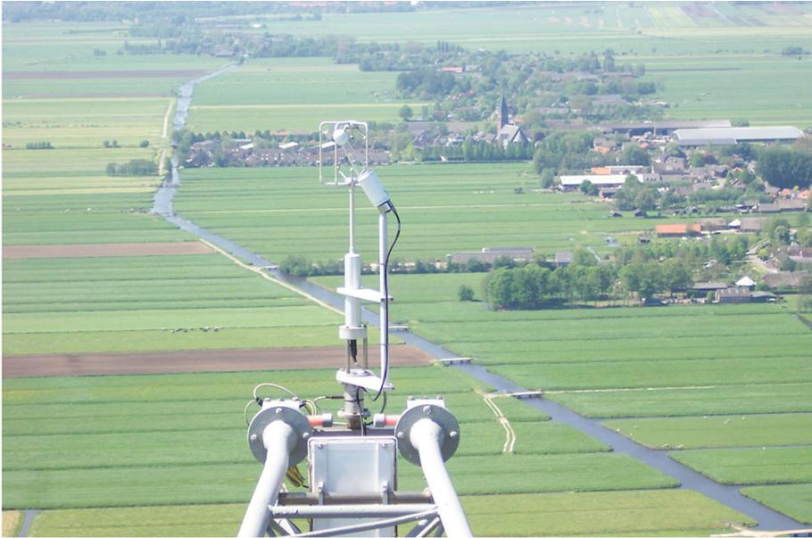
**Fig. 2** View to the south-west with turbulence instruments for measuring regional-scale fluxes of momentum, sensible and latent heat, and carbon dioxide. (Photo by Fred Bosveld)
