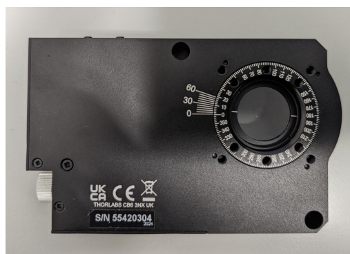
Figure 5.17: Rotation mount with mounted wire-grid polarizer.
