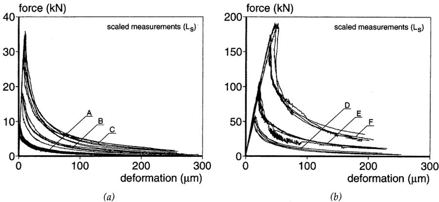
Fig. 3. Overview of the force-deformation curves for specimens A, B, C (a) and D, E, F (b) (DRY series).
