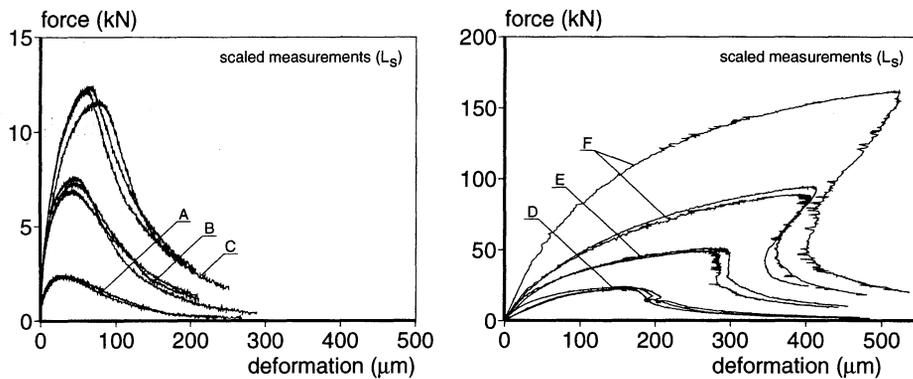
Fig. 6. Overview of force-deformation curves for the sandstone specimens.
