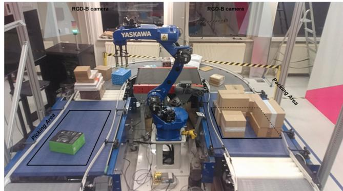
Fig. 1: Illustration of the real-world testing scenario. The system consists of a robotic arm for picking and packing items, a conveyor belt to feed incoming items, and RGB-D cameras mounted above to capture the packing scene and incoming item data.
