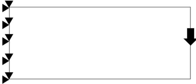
Figure 5.13: Boundary conditions for the flat composite plate: load case 1.
