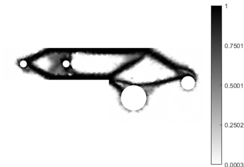
Figure 5.30: Chair bracket comparative analysis: topology optimization, volume fraction = 0.3.
