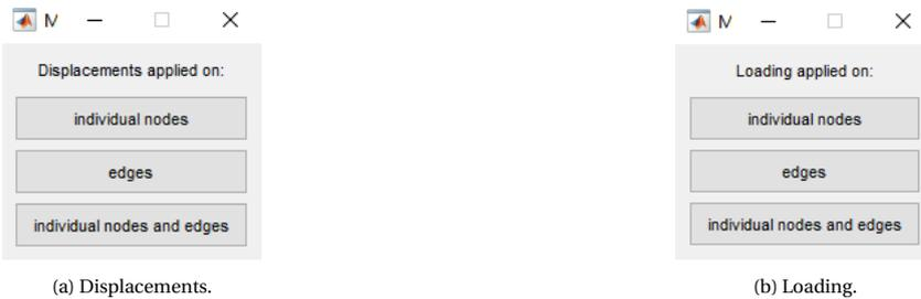
Figure 4.10: Menu for the application of the boundary conditions.
