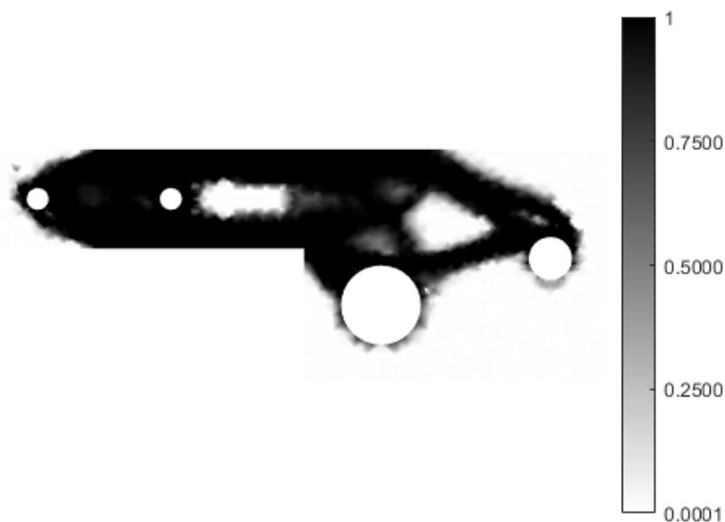
Figure 5.33: Chair bracket comparative analysis: topology optimization, volume fraction = 0.5.
