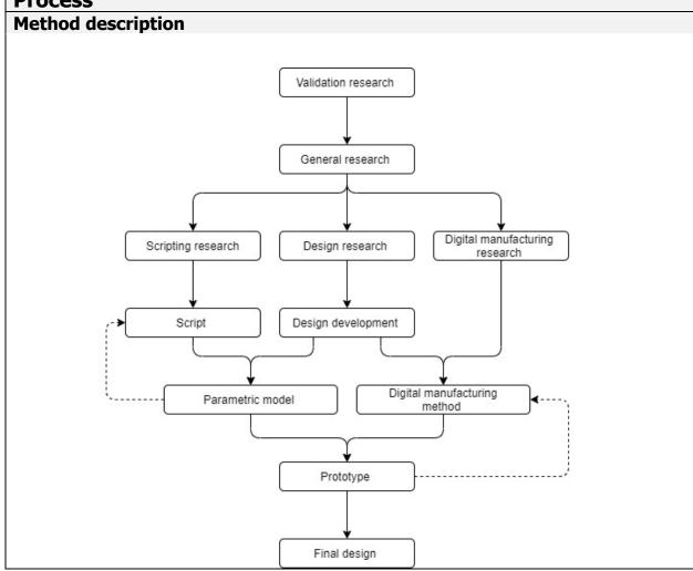
The research starts with a validation study to see if there is enough waste wood that can be reused as a building material in the Netherlands. The general research consists of obtaining knowledge about waste wood processing methods in the Netherlands. After the general research there will three parallel studies with the topics; scripting, design & digital manufacturing.
