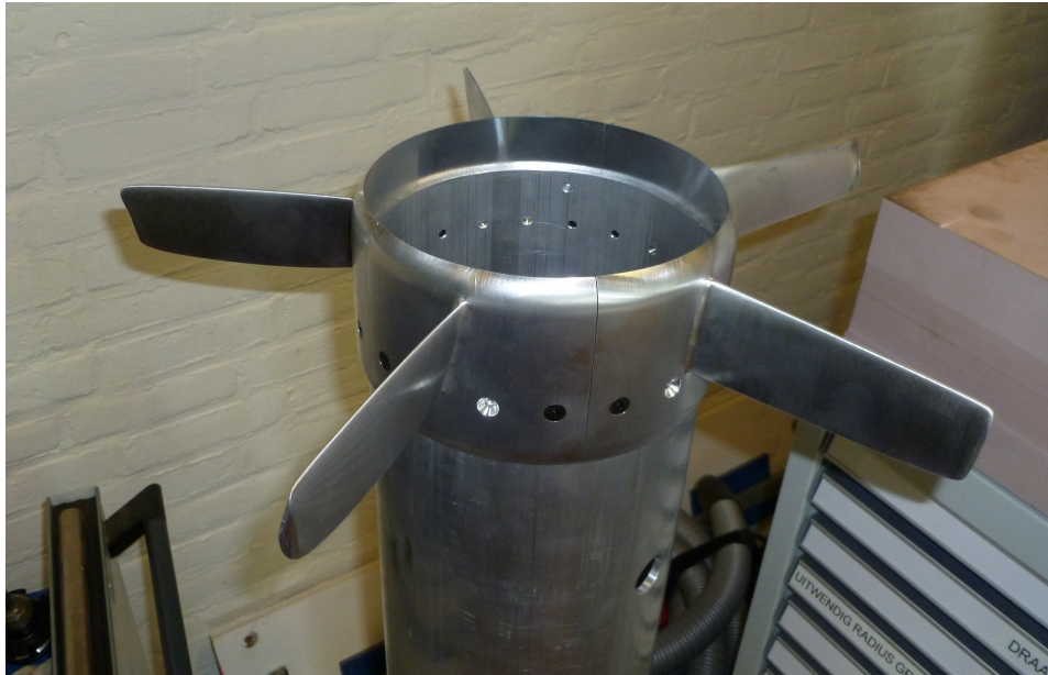
Figure 4.30: Finished stator in the workshop, front side shown. The chamfered flange leading edge and bolted connections can clearly be seen. The support tube is 180\text{mm} in diameter. Photo by author.
