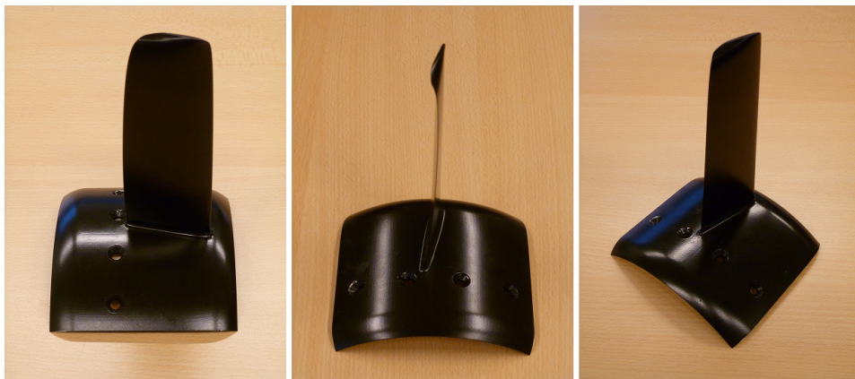
Figure 4.31: Three views of a completed stator blade with hub, painted in anti-reflective paint for PIV measurements. The middle image clearly shows how the twist near the root and tip gets quite large. The blade is located on the upstream part of the hub.
