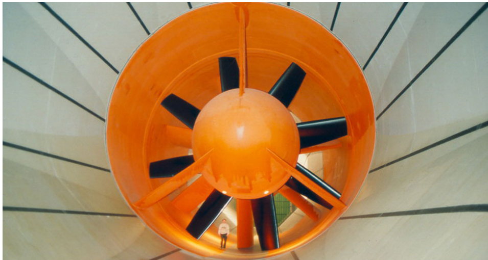
Figure 4.16: The fan of the LLF wind tunnel. Note the person standing at the bottom of the fan for scale. Taken from DNW website [29].
