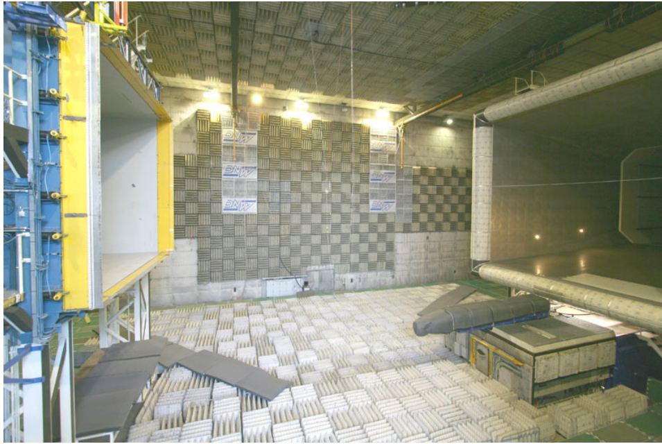
Figure 4.15: The open jet test section of the LLF wind tunnel. Taken from DNW website [29].
