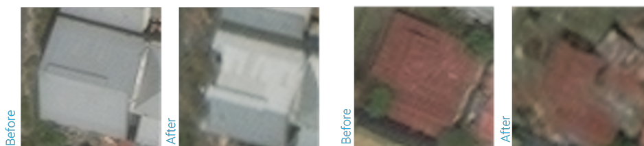
Figure 5.9: Visualisation of Major damage labelled polygons and classified with the No damage class (Example: Left Tsunami Palu 59-47 Right Tsunami Palu 60-225)
