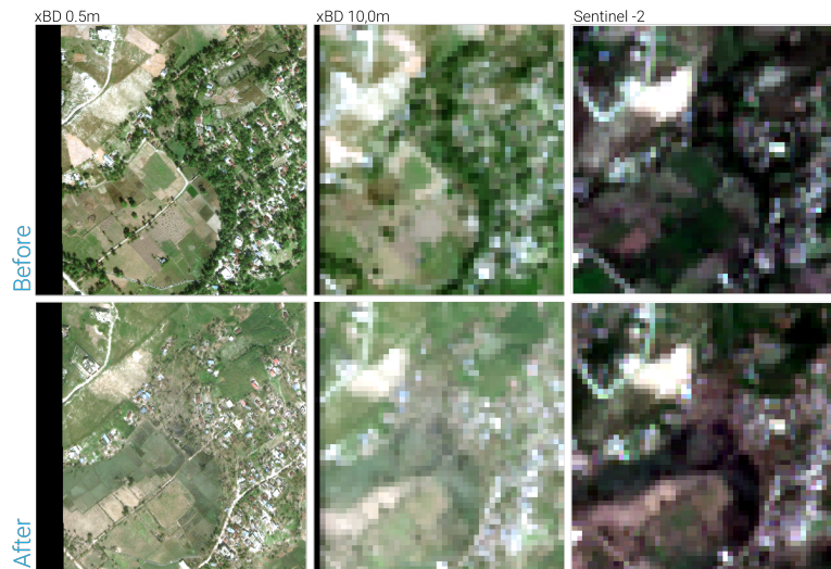
Figure 3.7: The comparison of an extracted Sentinel-2 1C image with the xBD 0.5 and 10.0-meter resolution visualisation (Example: Hurricane Matthew 03)
