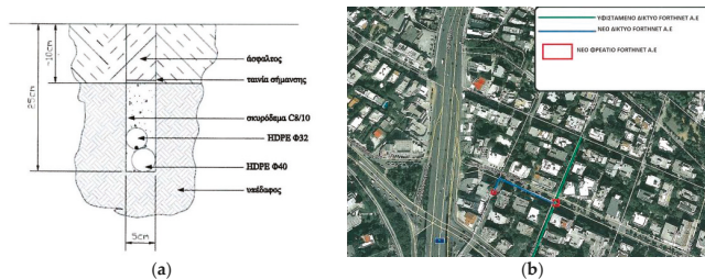
Figure 1. Documentation submitted for granting rights of way for public utilities. (a) Typical cross section; (b) location of network lines on drawing [23].
