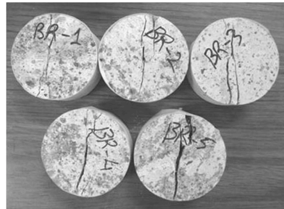
Fig. 7. (a) Comparison of experimental and numerical results of axial and lateral strain in the monotonic Brazilian test on sample BR-3. (b) Sample BR-3 after failure under monotonic loading in the experiment. 1
