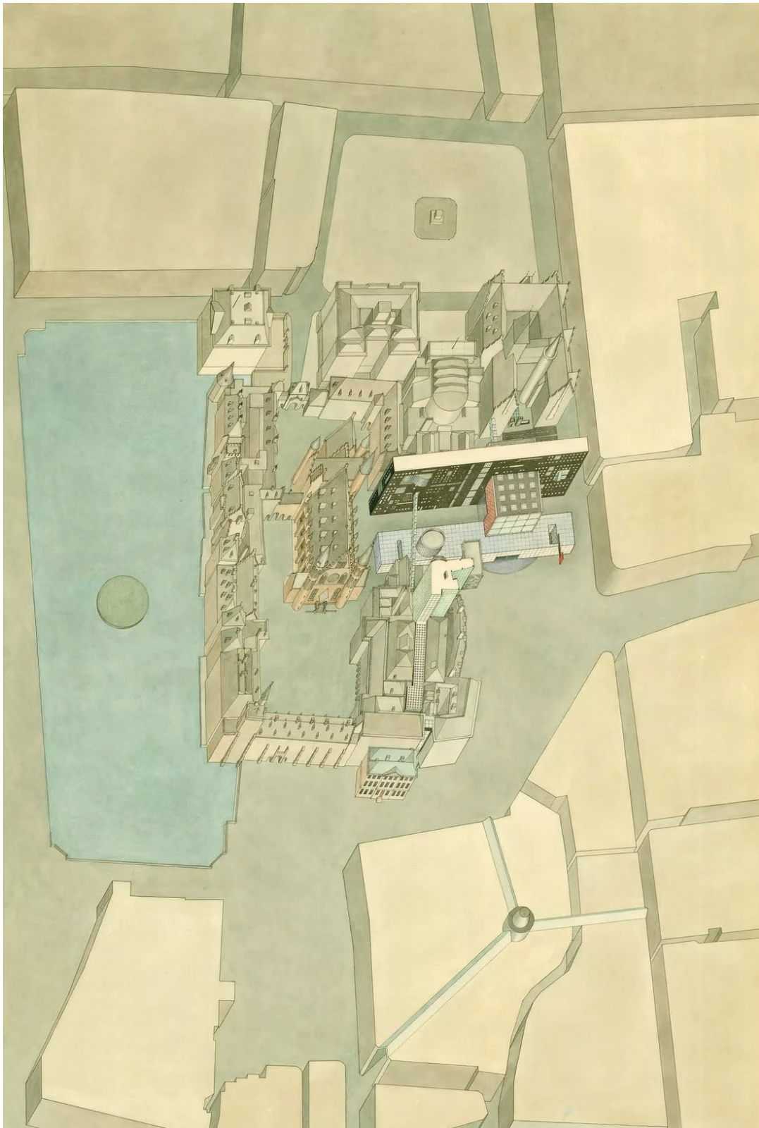
Fig 10. The OMA's drawing of their proposal of the Extension of the House of Representatives, which strikes through the Binnenhof and expose the Ridderzaal to the public through the negative gap
