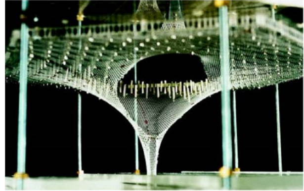
Figure 3. Suspension model for form-finding of the arches of the new train station in Stuttgart, Germany, 2000 ( https://www.pinterest.com/pin/317011261243639594/ ).
