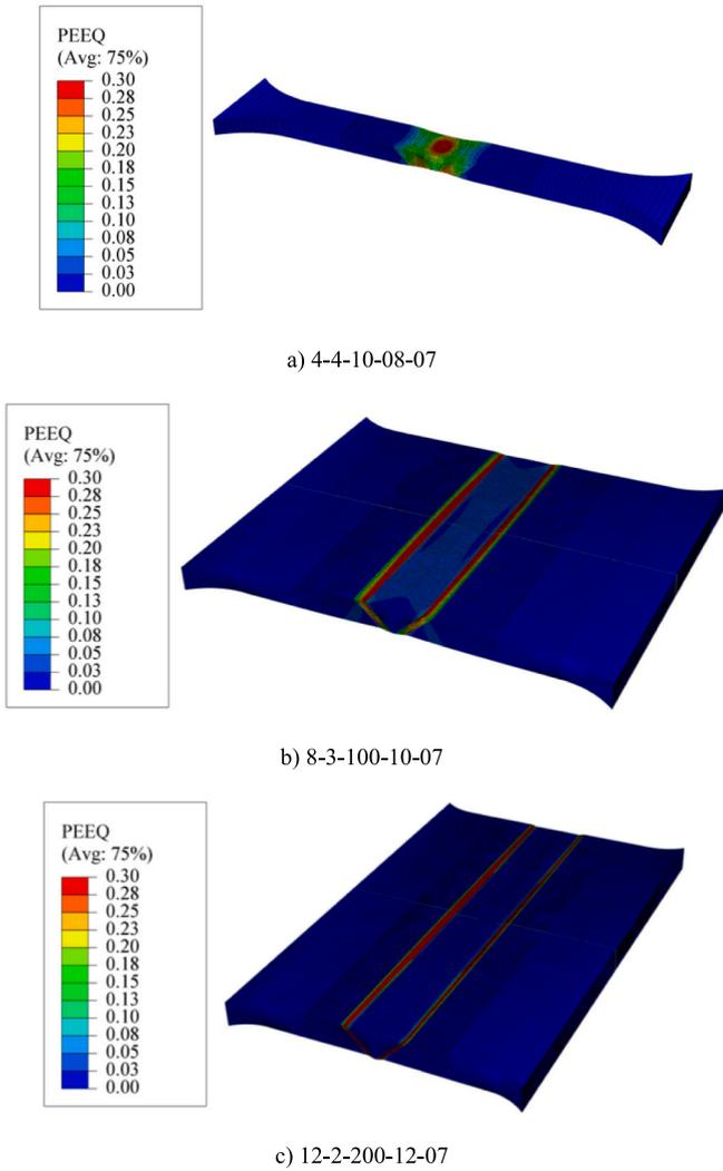
Fig. 6. Necking location in three FE models.
