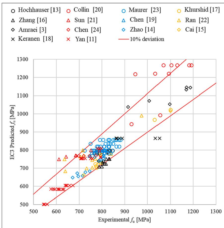
Fig. 12. EC3 prediction vs. experiments in literature.
