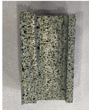
Figure 3.22: Sample Preparation for ARAMIS
