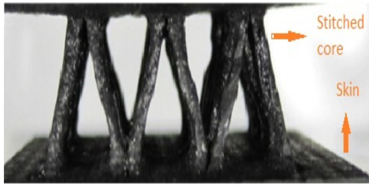
Figure 2.2: C/SiC composite sandwich structure with stitched lattice core lattice
