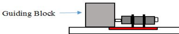
Figure 3.36: Core dipped in the Joining Paste (Red)
