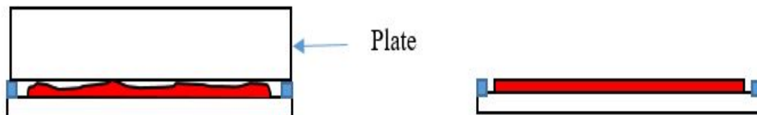
Figure 3.7: Uniform distribution of the joining paste
