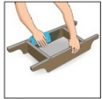
1. Wet the inside of a brick mould
