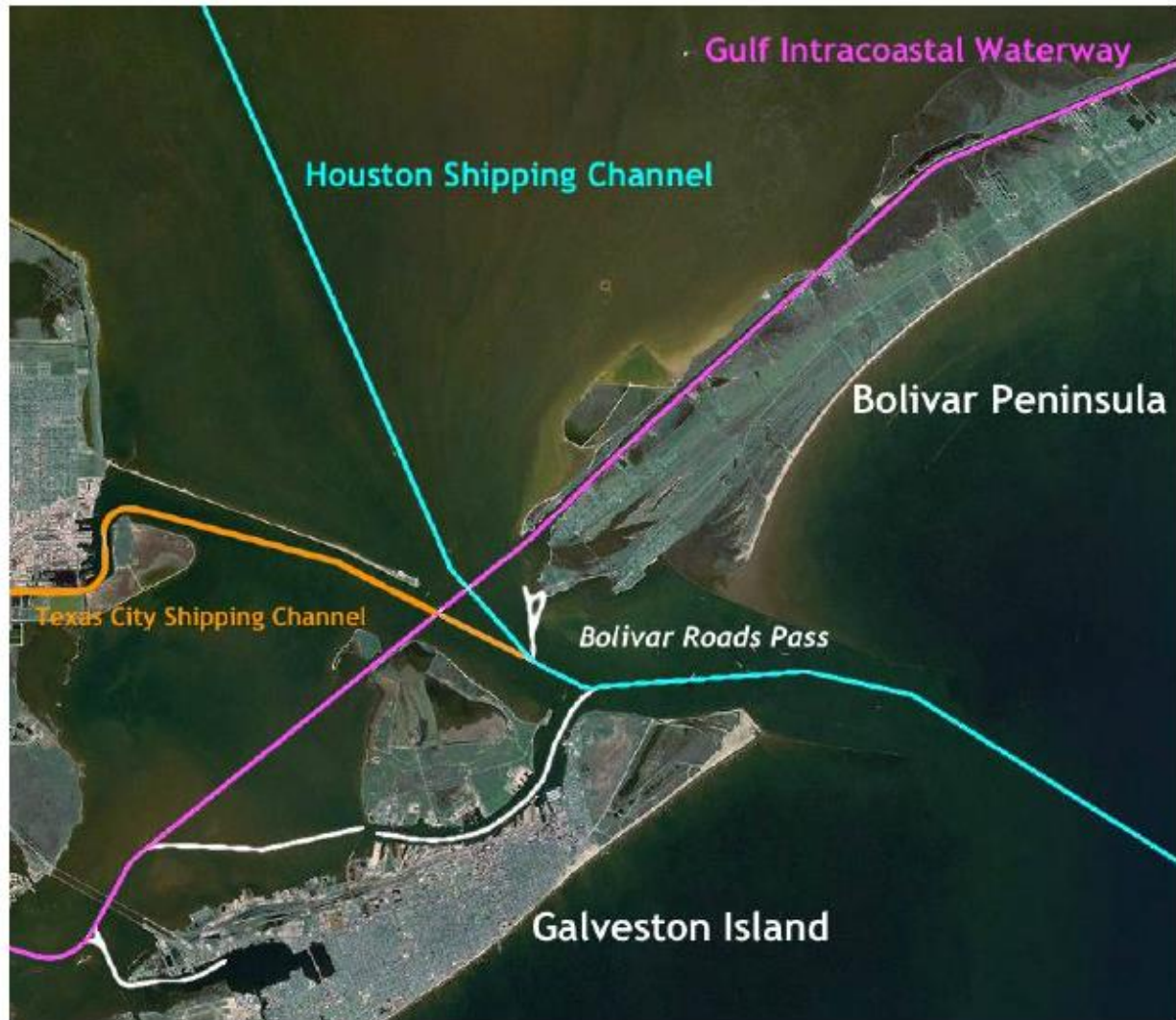
Figure 2-12: Navigational routes in the Galveston Bay Area [11]
