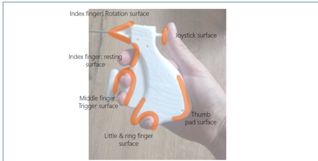
Figure 36. Second generation basis & necessary contact surfaces
