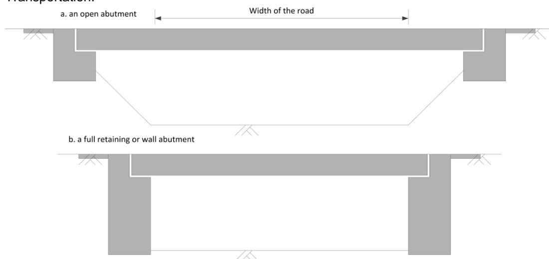
Figure 2-9 Common types of abutments
