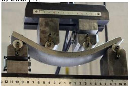
Figure 5-8 ECC plate in four-point bending test
