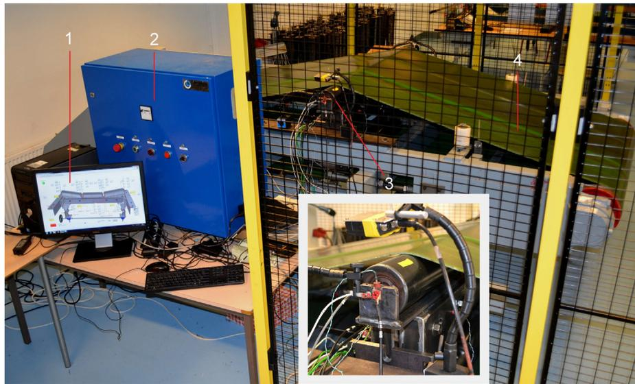
Fig. 1. The test rig. Note: 1 is data acquisition system, 2 is control box, 3 is idler frame, 4 is belt conveyor.
