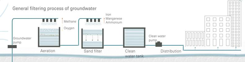
[Fig. 4.1]: Filtering process of groundwater to drinking water Source: own image
