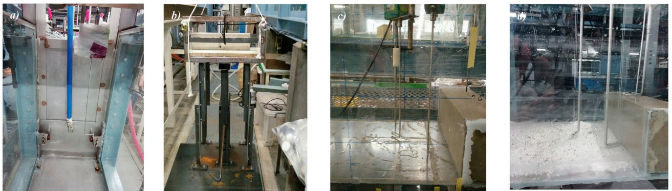
Fig. 4. Experimental Apparatus. a) View of the back of the gate. b) Weight system to release the gate. c) Wave gauge and velocity meters (smooth flat bed). d) Stone flat bed.
