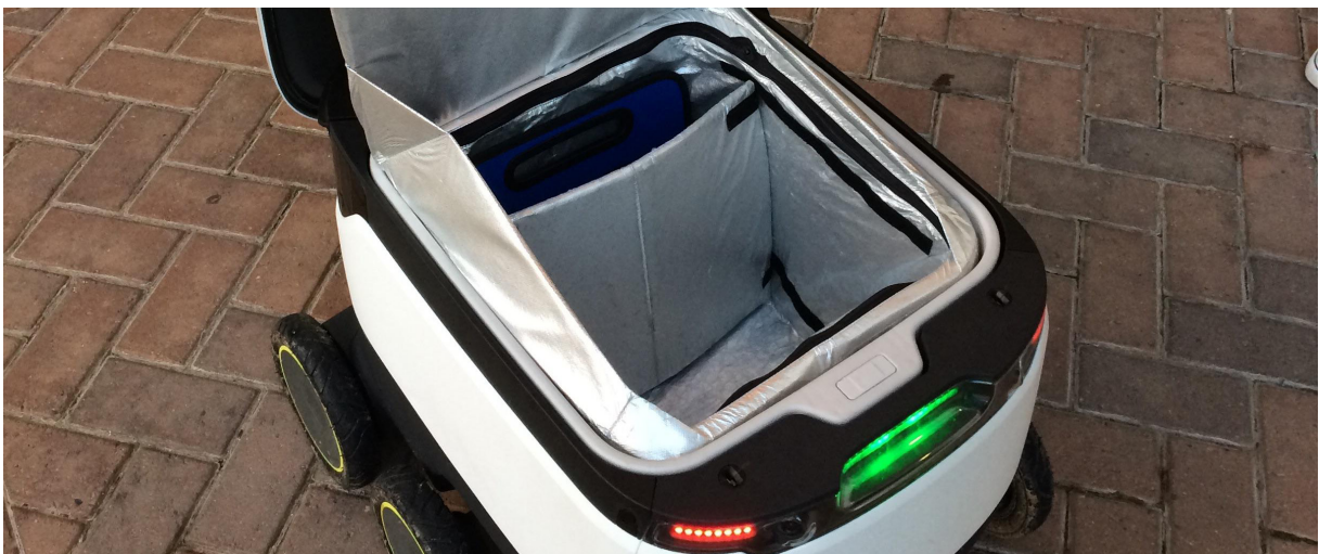
Figure 42. Thermal insulation as can be found in a Starship 'hot meal' delivery robot.
