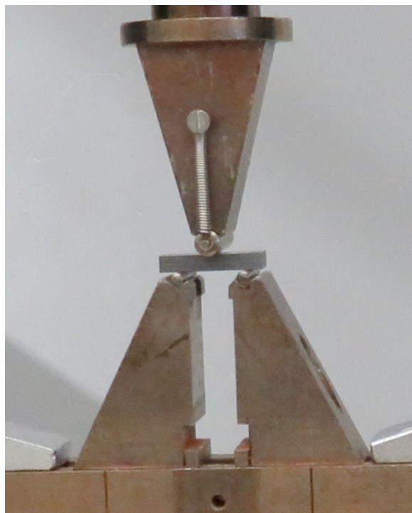
Figure C.3: The ILS test set-up.
