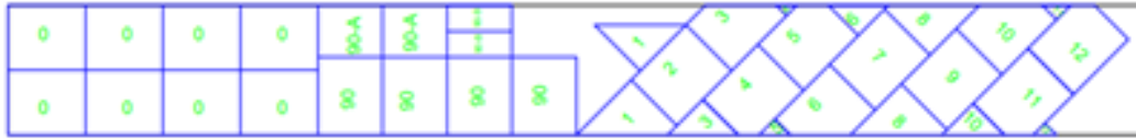
Figure B.2: The cutting layout of the prepreg.
