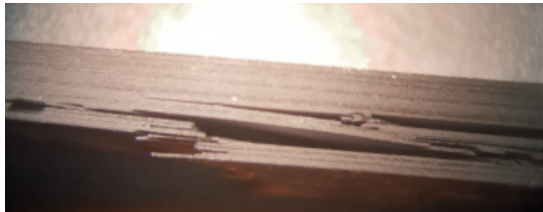
Figure 5.5: A close-up of a failed specimen with a tension failure mode.
