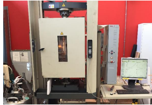
Figure 5: The TTM is shown with the climate chamber enclosing the load cell. A liquid nitrogen tank (bottom left) hooks up to the rear of the machine; temperature controls regulate the temperature within the chamber for testing.
