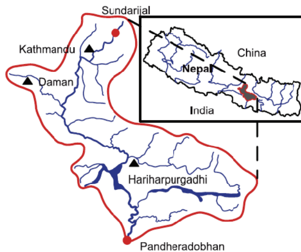
Figure 1-3. Location map of the Bagmati catchment in Nepal, triangles denote the rainfall stations, and circles denote the discharge gauging stations.
