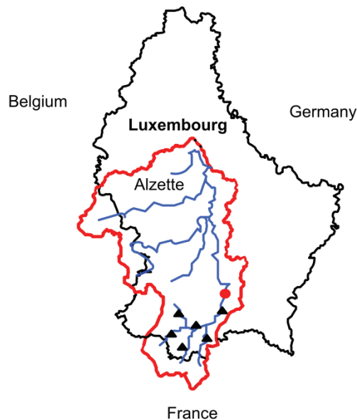
Figure 1-2. Location map of the Alzette catchment in Luxembourg, black triangles denote the rainfall stations, and circles denote the discharge gauging stations.
