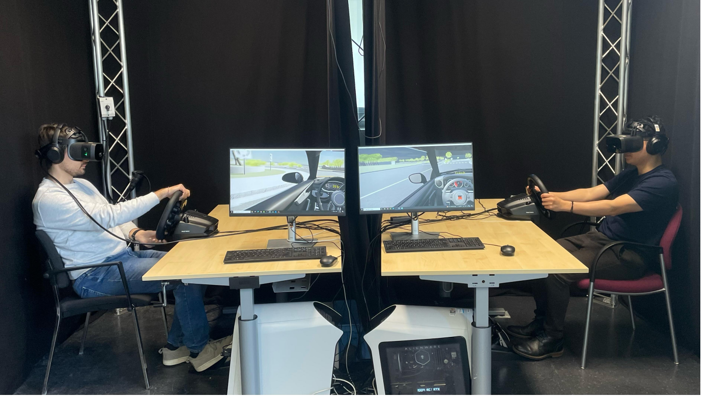
Figure 4: Experimental setup depicting two participants seated facing opposite directions, separated by curtains to prevent visual contact. Each participant had access to a steering wheel and gas and brake pedals positioned directly in front of them. Participants wore Varjo Base headsets and noise-cancelling headphones throughout the experiment. Both participants' views were continuously monitored through separate displays to ensure proper system functioning and participant compliance.
