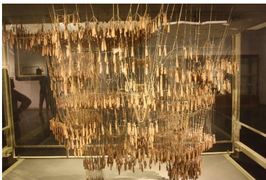
Figure 6: Hanging chain model of Sagrada Familia by Antonio Gaudi. (Photo: Steve Baskin)
