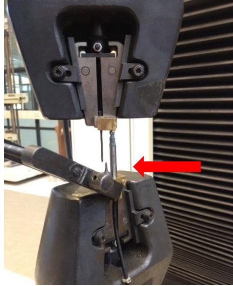
Figure 44: External sensor to measure the elongation.
