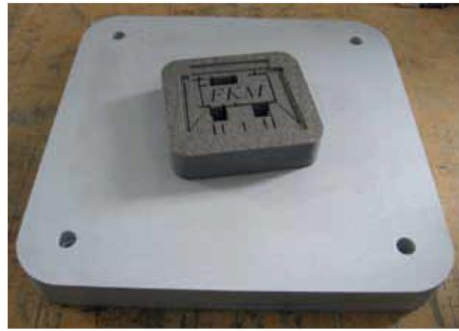
Figure 33: LaserCusing makes use of substrate plates which can be mounted in CNC machines [21].
