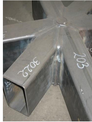
Figure 37: Mock-up of the joint. ©Arup
