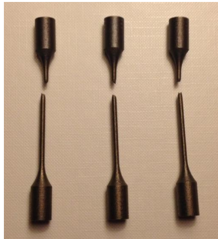
Figure 50: Ruptured test pieces.
