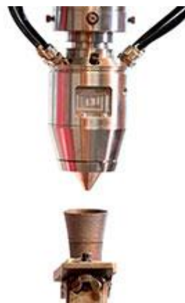
Figure 41: A CLAD machine building up an object. ©Réalisation 2013
