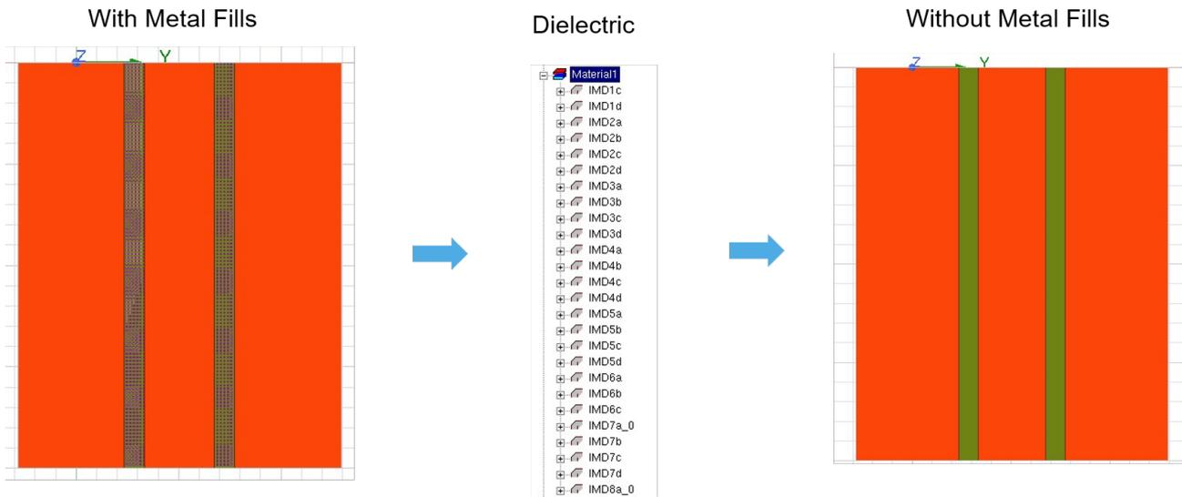
Figure 3.17.: Step 9 - Placing the epsilon effective parameters in dielectric layers
